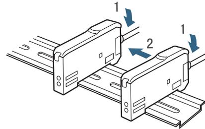
Note: For vibration may disconnect the connection. Please use the optional installation accessory (PFP-M) for securing. Please remove it in the reverse sequence. Make sure that the amplifier unit should be removed before DIN track is removed.
