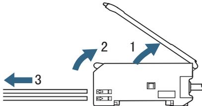
Note: To protect the characteristics of the optical fibers, please confirm whether the locking status is unlocked before pull out the optional fibers.
