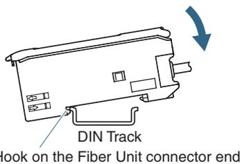
Note: Make sure that the insertion side of the optical fiber unit is mounted onto the track before carrying out the installation. Reverse installation will reduce the installation strength.
