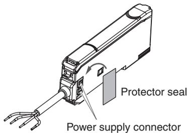
Make sure that the power supply is turned off before separating or adding amplifiers.
