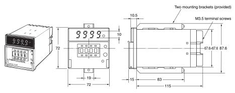
Note: 1. The panel cutouts for the H5AN are as shown (according to DIN437000).
