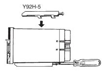
After attaching the mounting brackets, turn the screws clockwise to tighten them sufficiently. When the screws are completely tightened, you will hear the threads disengage.
