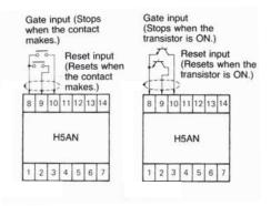
When connecting a transistor circuit not of the open collector type to the gate or reset inputs as shown below, the voltage of the transistor circuit (+V) should be 13 to 30 V, and the  $V_{\text{CE(S)}}$  of the transistor should be less than 3 V (the current that flows from either terminal 9 or 10 is approximately 10 mA). Moreover, it is essential that the circuit be ON for gate or reset input, and OFF when there is no input.
