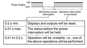
Note: Use a Timer with power failure backup memory (models ending with -M) and enable memory backup if holding the status before the power failure is required when the power is interrupted.
