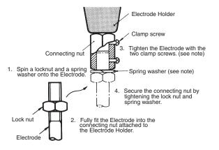
Note: Clamp screw and spring washer are not provided for the BS-1T Electrode Holder (titanium, HAS B, or HAS C).
