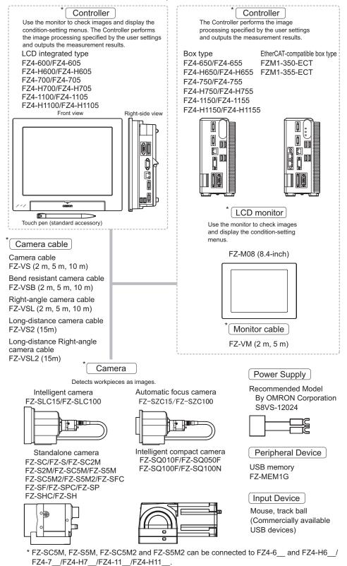
\* Intelligent compact camera can be connected to FZ4-6\_\_ and FZ4-H6\_\_/FZ4-7\_\_/FZ4-H7\_\_/ FZ4-11\_\_/FZ4-H11\_\_.
