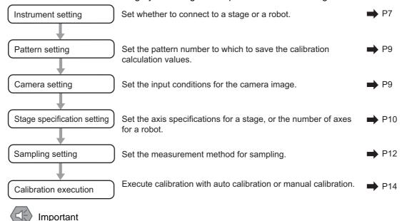
Pattern-specific setting data and created calibration parameters are all retained as part of scene group data.
