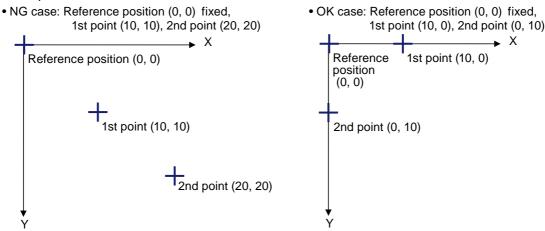
After sampling is complete, the calibration values are registered by the [Calibration calculation] command.
