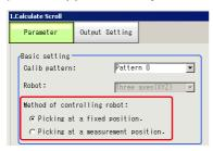
The above setting varies depending on the stage "after the workpiece is grabbed until it is moved" in which position adjustment is performed.
