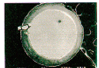
Magnified photograph of a diode short-circuit
