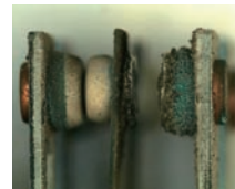
Corrosion due to nitric acid
