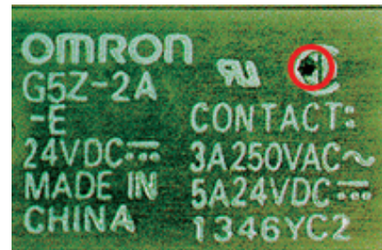
Hole made in a case by a relay terminal
