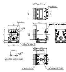
\* The base at the bottom of the camera can be mounted to the bottom, top, and both sides. Remove the base mounting screw (M4x8) and correct the mounting position. (Recommended mounting screw torque: 1.2 N·m)
