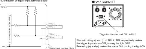
\*Current flowing through the short circuit is less than 2mA.
