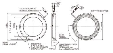
Tightening torque: 0.54N · m
