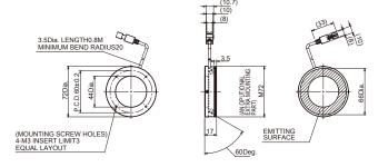
Tightening torque: 0.54N · m
