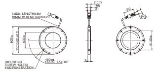
Tightening torque: 0.54N · m
