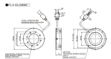
Tightening torque: 0.54N · m
