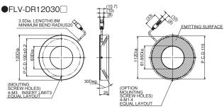
Tightening torque: 0.54N · m
