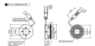
Tightening torque: 0.54N · m
