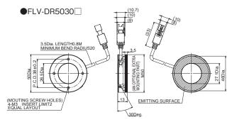
Tightening torque: 0.54N · m
