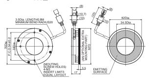
Tightening torque: 0.54N · m
