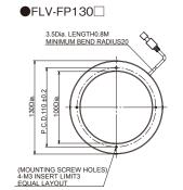
(MOUNTING SCREW HOLES) 4-M3 INSERT LIMIT3
