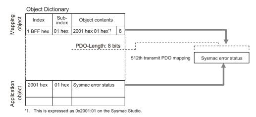
In the previous example, a single application object is assigned to the PDO at index 1BFF hex (name: 512th transmit PDO mapping). This PDO is a TxPDO. The application object contains the Sysmac error status at index 2001 hex and subindex 01 hex.
