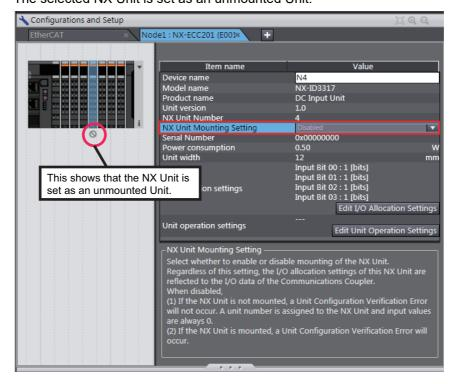
To change an NX Unit that is set as an unmounted Unit to a mounted NX Unit, set the NX Unit Mounting Setting to Enabled in step 2.
