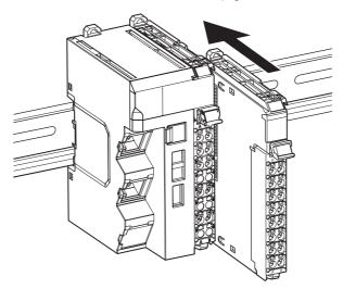
**3** Press the NX Unit with a certain amount of force against the DIN Track until you hear the DIN Track mounting hook lock into place.
