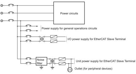
Power Supply System Diagram
