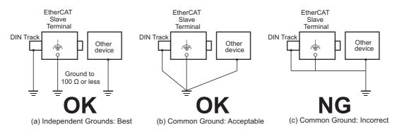
If the DIN Track is made of steel and the surface is not treated to produce an insulating material, you can omit grounding the functional ground terminal on any Unit that has one, as shown in the following figures.
