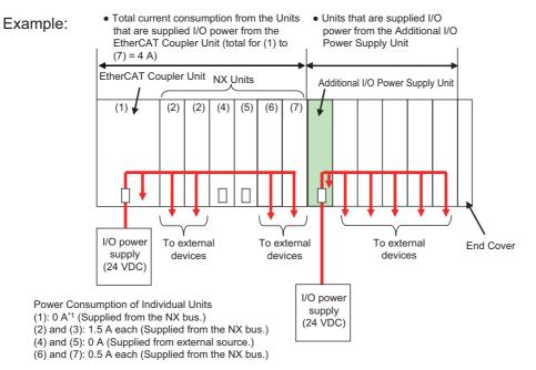
\*1. The current consumption of the EtherCAT Coupler Unit is not actually 0 A. However, a value of 0 A is used in this calculation example.
