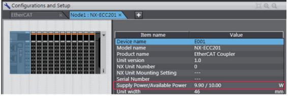
If the power to supply exceeds the NX Unit power supply capacity of the Unit that is selected to supply the NX Unit power, a yellow warning icon is displayed by the first NX Unit for which there is not sufficient capacity and also by all the remaining NX Units.
