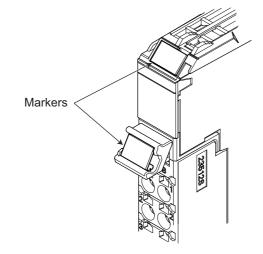
The marker attachment locations on the NX Units depend on the type of external connection terminals. Refer to the user's manual for the NX Units that you will use for the marker attachment locations.
