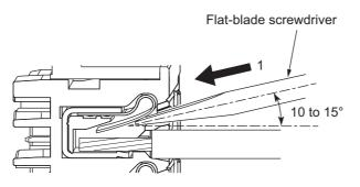
**2** Leave the flat-blade screwdriver pressed into the release hole and pull out the wire.
