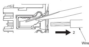
**3** Remove the flat-blade screwdriver from the release hole.
