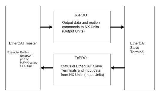
The EtherCAT application layer can hold more than one object to enable the transfer of various process data of the EtherCAT Slave Terminal.
