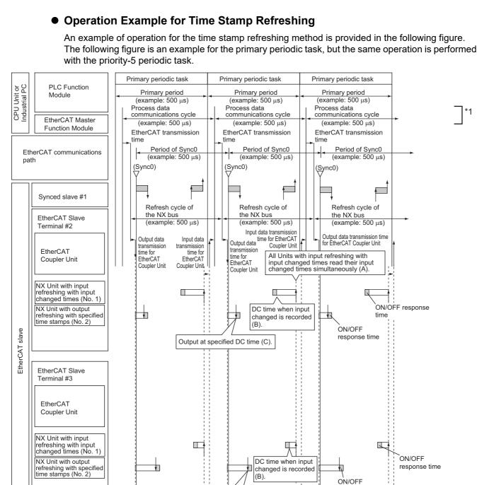
\*1. For a built-in EtherCAT port that can perform process data communications with a Slave Terminal in more than one periodic task, this is called process data communications cycle 1.
