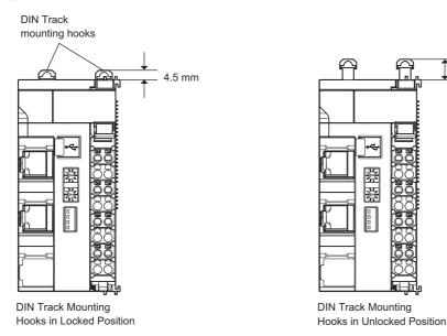
If the DIN Track mounting hooks are pressed down, they are in the locked position.
