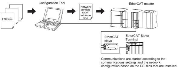
ESI files for the EtherCAT Coupler Unit and NX Units can be downloaded from the OMRON website.
