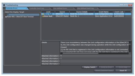
2 In the Select the Display Target Area of the Controller Event Log Tab Page, select the Units to clear and click the **Clear** Button.
