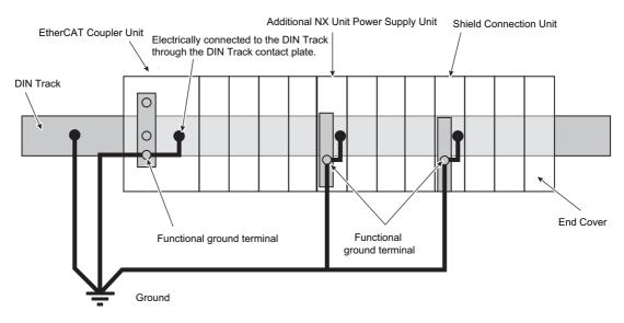
If the DIN Track is made of steel and the surface is not treated to produce an insulating material, you can omit grounding the functional ground terminal on any Unit that has one, as shown in the following figures.
