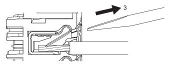
After you make a connection, lightly pull the twisted wire or the solid wire to make sure that the wire is securely connected to the terminal block.
