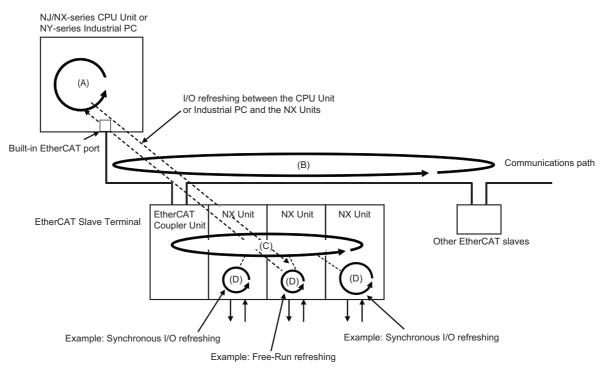
This section describes the operation of the NX Units on the EtherCAT Slave Terminals and the operation of I/O refreshing with the various series of CPU Units or Industrial PCs using the letters given in the above figure.
