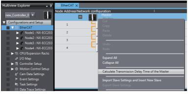
**2** The transmission delay times of PDO communications cycle 1 and PDO communications cycle 2 are displayed in the Output Tab Page.
