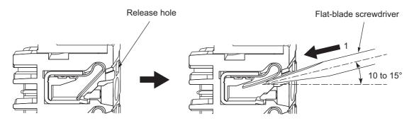
2 Leave the flat-blade screwdriver pressed into the release hole and insert the twisted wire or the solid wire into the terminal hole.
