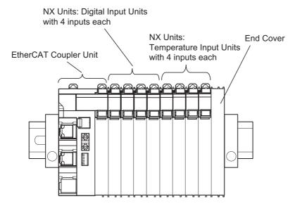
The widths of the Units in the example EtherCAT Slave Terminal configuration and the total configuration width are given below.
