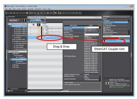
**3** Select the EtherCAT Coupler Unit on the EtherCAT Configuration Edit Tab Page.
