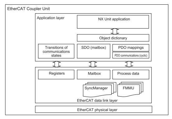
The following figure shows how the CoE is structured for an EtherCAT Coupler Unit.
