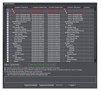
**2** To transfer the Unit operation settings for the EtherCAT Slave Terminal and the application data for the NX Units, make the setting to transfer the Slave Terminal Unit operation settings and NX Unit application data in the Synchronization Pane.
