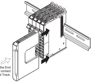
Press in until the End Cover comes into contact with the DIN Track.
