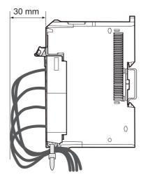
**3** Bundle the wires with a cable tie and secure them to the screwless clamping terminal block.
