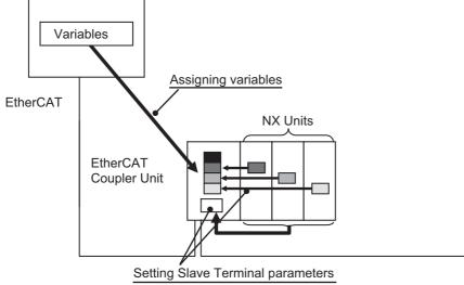
Make the above settings on the Sysmac Studio. Then connect the Sysmac Studio to the CPU Unit or Industrial PC and transfer the settings to the CPU Unit or Industrial PC and to the Slave Terminals.
