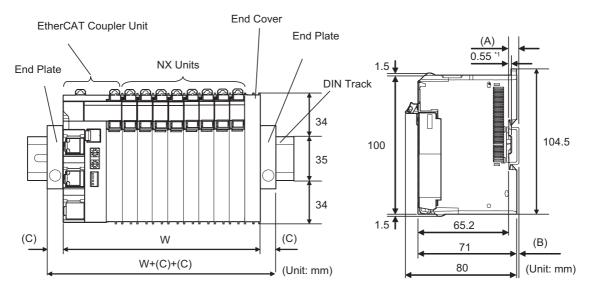
\*1. The dimension is 1.35 mm for Communications Coupler Units with lot numbers through December 2014 or for NX Units with 12-mm widths with lot numbers through December 2014.
