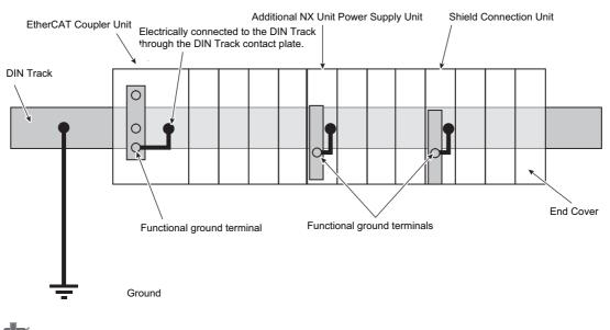
■ DIN Track Made of Steel and Surface Not Insulated
