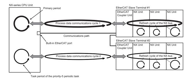
The (D) refresh cycles of the NX Units depend on the I/O refreshing method of each NX Unit. You can also use NX Units with different I/O refreshing methods together. Refer to 10-3 I/O Refreshing for EtherCAT Slave Terminals on page 10-8 for information on the I/O refreshing methods of each NX Unit.
