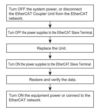
This section describes how to replace the EtherCAT Coupler Unit.
