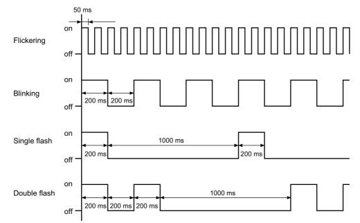
The timing of indicator flashing is given below.
