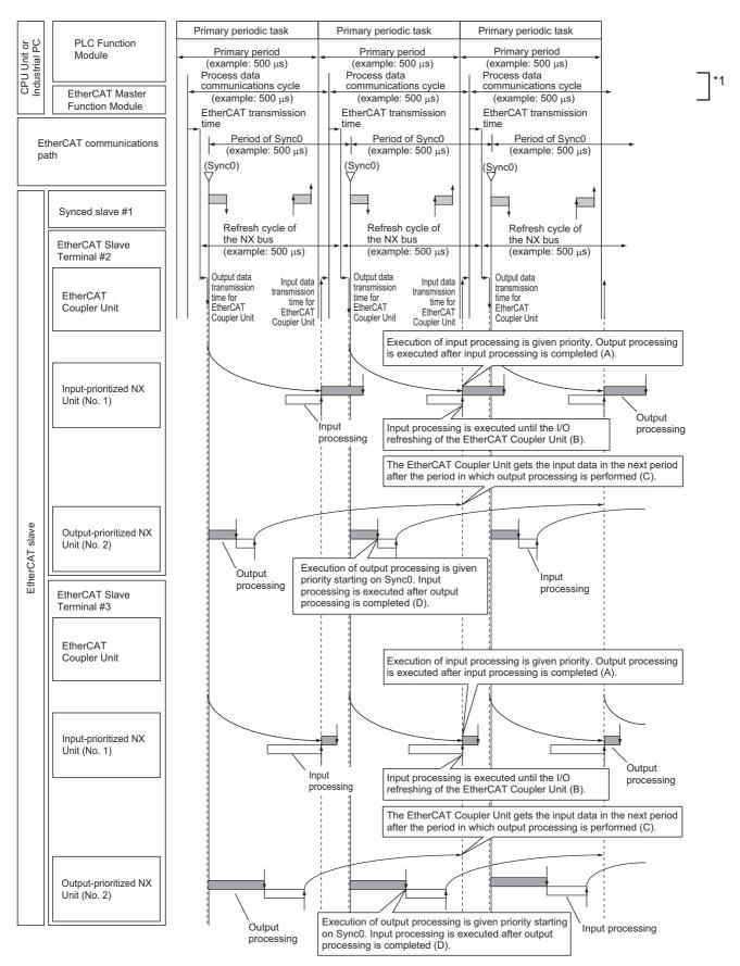
\*1. For a built-in EtherCAT port that can perform process data communications with a Slave Terminal in more than one periodic task, this is called process data communications cycle 1.
