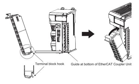
Mount a terminal block that is applicable to the model of the EtherCAT Coupler Unit. Refer to *4-5 Terminal Blocks* on page 4-14 for the applicable terminal blocks.
