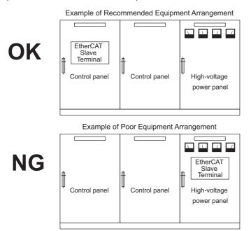
Examples of Equipment Arrangement in Panel with High-voltage Devices
