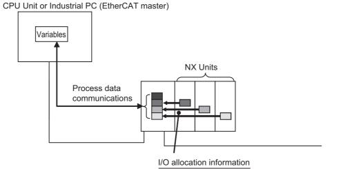
The EtherCAT Coupler Unit and the NX Units contain default values for the I/O allocation information. These default values are sufficient for a standard exchange of I/O data. Change the settings as necessary.
