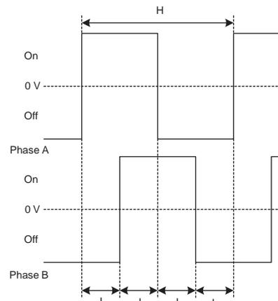
Counter Input Z\* / Digital Inputs (24 V)
