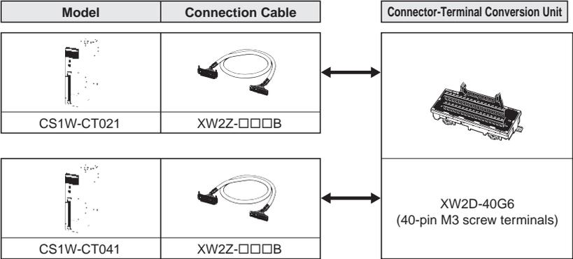
**Note:** 2 units are required for 4 axes control.
