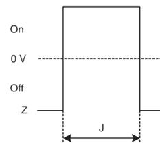
\* Maximum allowed frequency of Z-pulses is 1 kHz
