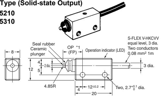
M16 Type (Contact Output/Solid-state Output)
