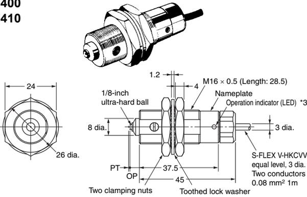
M16 Type (Contact Output/Solid-state Output)
