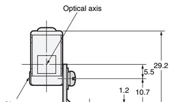
\*The Mounting Bracket can be attached to side A.
