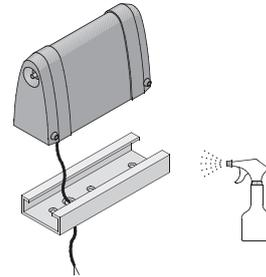
7. Safety edges with a C-base (SGE-365) have to be clipped with one side into the mounting base. Then press in the complete c-base. Pulling or pushing the safety edge into the mounting base can cause damage to the safety edge and should be avoided at all costs.
