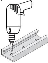
When using SGE-125, drill a pilot hole to the groove such that the head of a countersunk screw can go through (approx. 8 mm).
