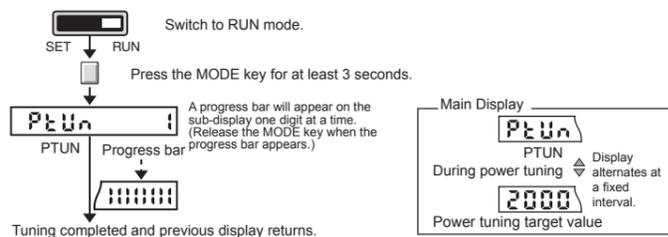
The power tuning target value can be changed. Refer to 5. Detailed Settings.
