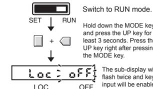
If a key is pressed while key operations are locked, "LOC ON" will flash twice on the display to indicate that key operations have been disabled.
