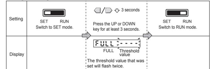
It does not matter whether or not there is a workpiece. The value that is set will depend on the detection method and power adjustment settings.
