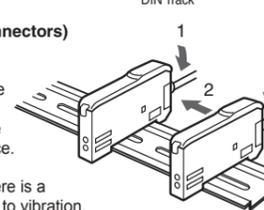
Secure the Units with an End Plate (PFP-M) if there is a possibility of the Amplifier Units moving, e.g., due to vibration.
