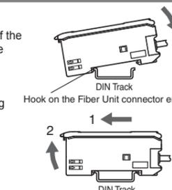
Always attach the Fiber Unit connector end first. If the incorrect end is attached first, the mounting strength will be reduced.
