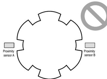
With this installation, both proximity sensors are turned OFF when the rotation of the cogwheel stops. If both sensors are turned OFF for more than 1 second, G9SX-LM□ will detect it as an error.
