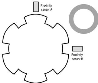
Install proximity sensors so that one of them is turned ON when the rotation of cogwheel stops. Install one proximity sensor on the center line of the concavity width, and the other on the center of the convexity width so that one of the proximity sensors will be turned ON when the rotation of the cogwheel stops.
