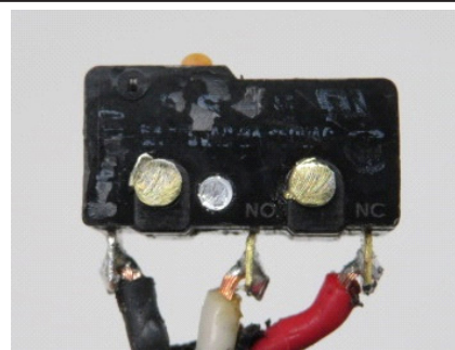
Enlarged view of contact of NC side (welded)
