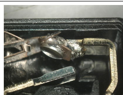
Enlarged view of contact of NC side (welded)
