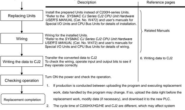
operation. If so, it is necessary to adjust cycle time in the PLC Setup.
