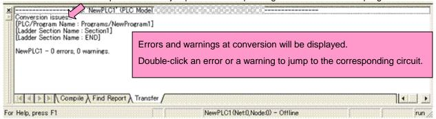
Some instructions cannot be converted. Modify the ladder program by referring to *Appendix A. Instructions* converted by Change Model on CX-Programmer.
