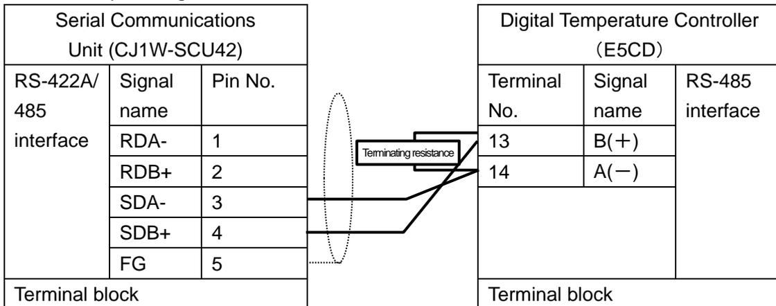
\*Connect 120 Ω (1/2 W) terminating resistance between B(+) and A(-) of the Digital Temperature Controller that is connected at the end of the network.
