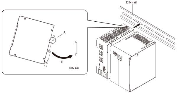
Push the rail stopper in the B direction, and then raise and lock it.
