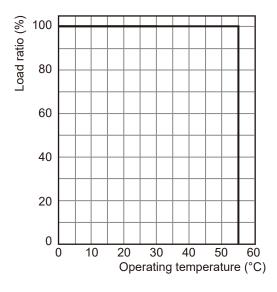
• Contact mounting (less than 15 mm space at the left and right)
