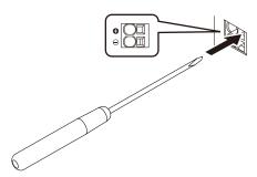
With the tip of the flat blade screwdriver in the hole, insert a cable into a round hole at the left of the terminal block.
