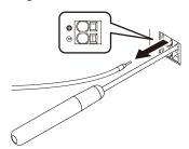
Pull out the flat blade screwdriver.
