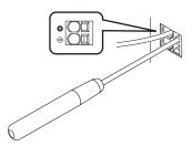
3 Pull out the flat blade screwdriver. Then, the cable is locked.
