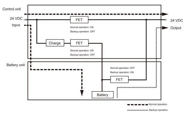
Note 1. In normal operation, 24 VDC is output as-is for charging the battery and from the input power supply. If the 24 VDC from the input power supply becomes lower, the operation automatically switches to backup operation, and 24 VDC is output from the battery.
