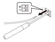
2 Pull out the flat blade screwdriver.
