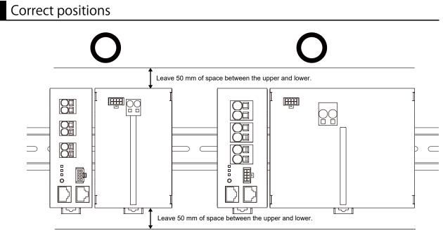
Note 1. This UPS can be mounted with the sides in close contact. Up to 3 units can be mounted in close contact. Follow the derating curve during mounting with the sides in close contact. For details, refer to A-2 Characteristic data on page A-5.
