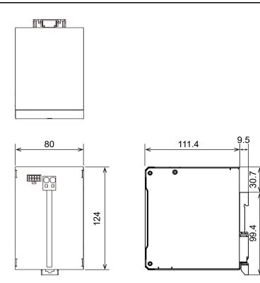
Note Unit: mm / Iolerance:±1mm
