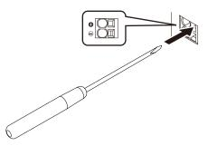
2 With the tip of the flat blade screwdriver in the hole, insert a cable into a round hole at the left of the terminal block.
