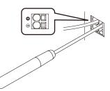
**3** Pull out the flat blade screwdriver. Then, the cable is locked.
