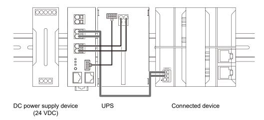
2 When using the UPS monitoring software or the I/O signal, connect the unit to the target device with a connection cable.
