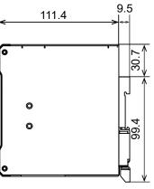
Note Unit: mm / Tolerance:±1mm
