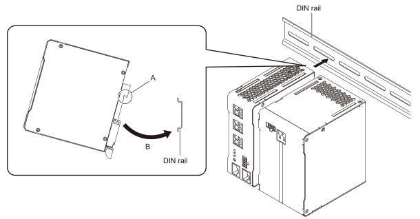
2 Push the rail stopper in the B direction, and then raise and lock it.
