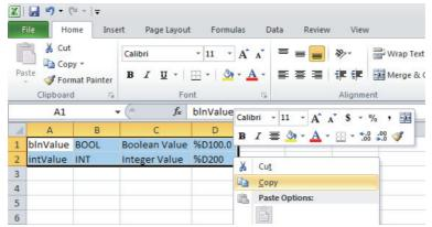
**3** Paste the variables in the device variable table of the HMI project.
