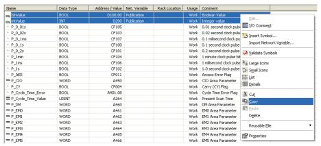
Paste the variables in the device variable table of the HMI project.
