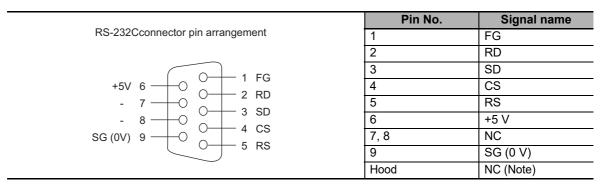
Note The hood will have the same electric potential as the connector hood of the connection destination.
