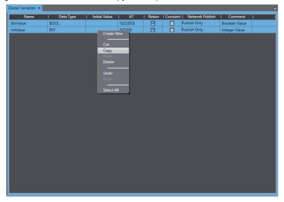
**2** Paste the device variables in a spreadsheet, delete unnecessary rows, and sort and copy the remaining rows. Refer to *A-1 Clipboard Format for Device Variable Table Data* on page A-2 for information on the order of the rows.
