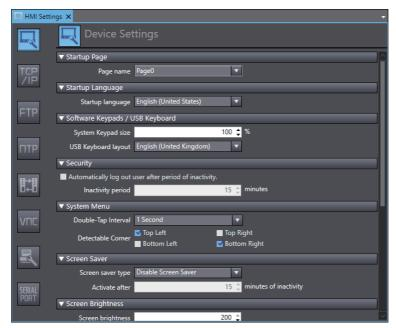
Click the Serial port settings Button and set the settings configured in CX-Programmer on the Serial port settings dialog box. Select Connection with external devices for application.
