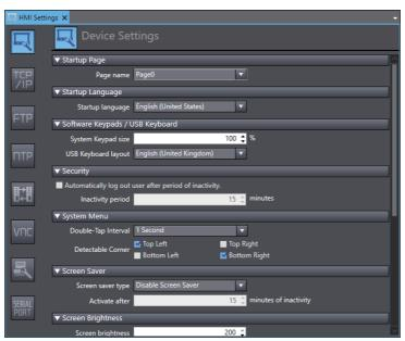
Click the TCP/IP Settings Button and set the IP address for Ethernet port 1 in the TCP/IP Settings. Also set the subnet mask and default gateway as required.
