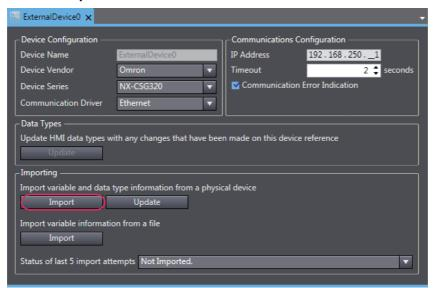
The global variables are transferred from the Controller and registered as device variables.
