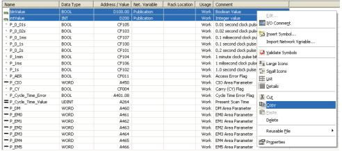
**2** Paste the variables in the device variable table of the HMI project.
