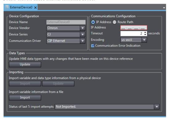
**3** Make the following settings for the external connected device.
