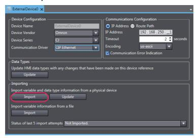
**3** The global variables of the CJ-series PLC are transferred and registered as device variables.
