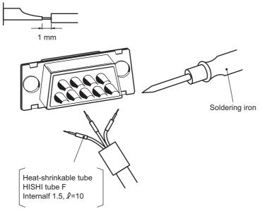
**4** Push the heat-shrinkable tubes back over the soldered joints, then heat them using a jetter to shrink them in place.
