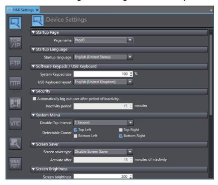
2 Click the TCP/IP Settings Button and set the IP address for Ethernet port 1 in the TCP/IP Settings. Also set the subnet mask and default gateway as required.
