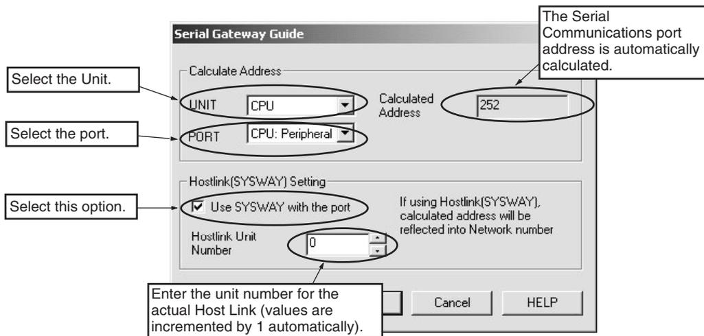
**Note** When using the CX-Programmer, enter the actual Host Link unit number. Do not add 1 to the value. The CX-Programmer will automatically add 1 internally.
