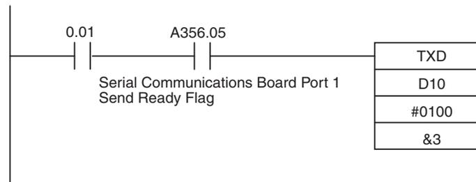
**Note** Use an AND of an NO condition of the Send Ready Flag (A356 bit 05/13) in the input conditions when executing the TXD instruction for a Board.
