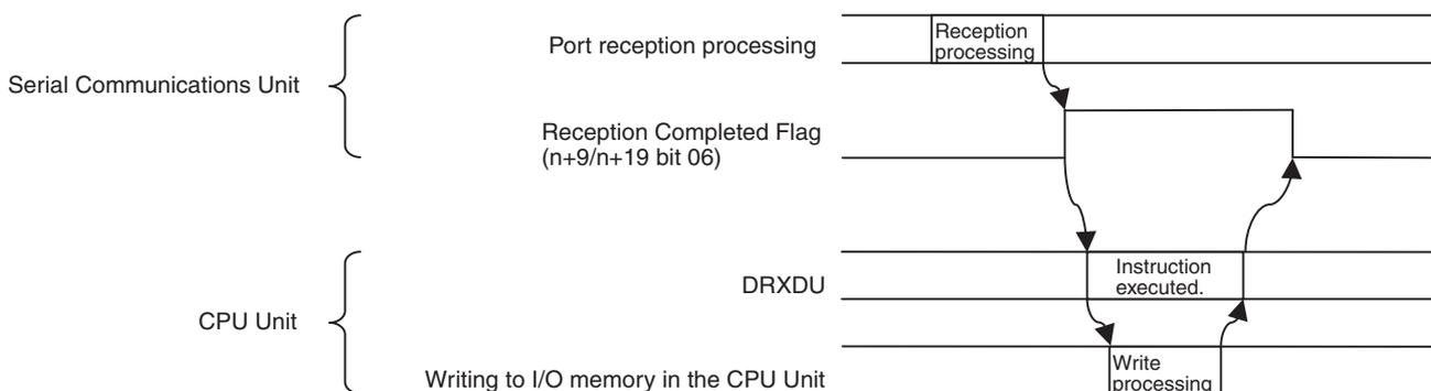
**Note** The DRXDU(261) instruction is executed immediately. Received data is therefore stored in I/O memory in the same cycle as the one in which the instruction is executed.
