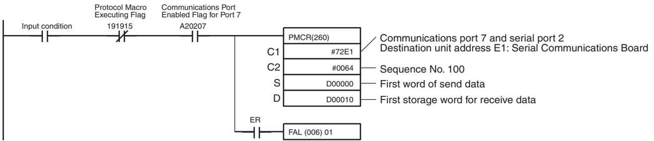
If the input condition turns ON when the Protocol Macro Executing Flag (CIO 191915 for port 2) is OFF and the Communications Port Enabled Flag (A20207 for internal logic port, communications port 7) is ON, communications sequence No. 100 registered in the Serial Communications Board is called, and data is sent and received via port 2 of the Serial Communications Board.
