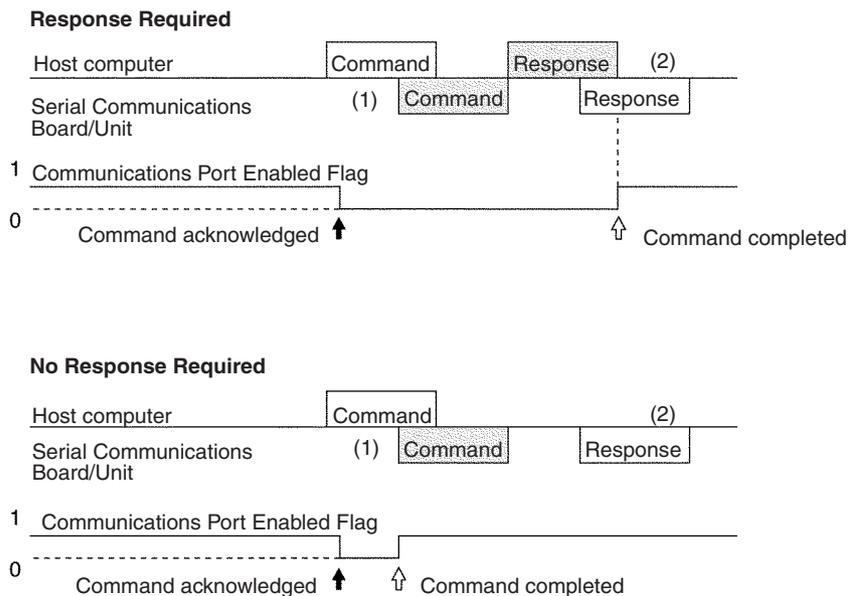
Command transmission to the host computer can start even when the port is receiving a command from the host computer (1). The transmission of a response to the command from the host computer is postponed until the transmission of the command to the host computer is completed (2).
