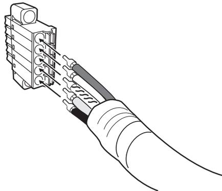
6. Connect the connector with the communications cable attached to it to the connector on the Unit. Then tighten the screws to secure the connector to the Unit.
