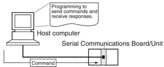
The host computer must be programmed to send the Modbus-RTU commands and receive responses.
