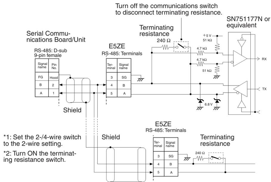
**Note** Terminal block pins 1 and 2 cannot be connected. If these blocks are used, operation of the E5ZE may fail.
