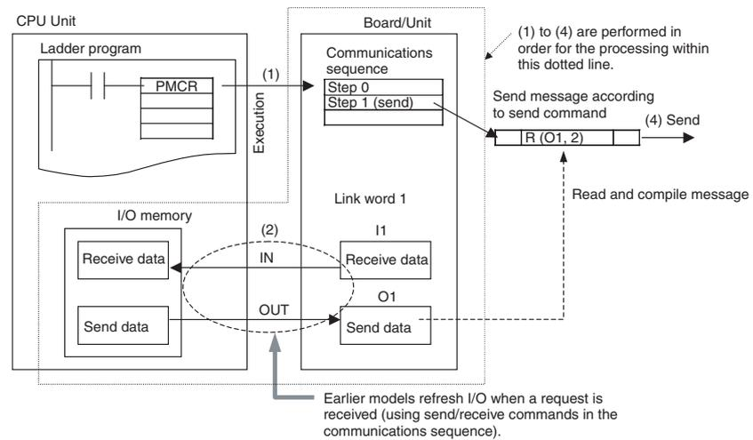
Therefore, when a send command is executed ((1) in the above diagram), the read processing of data using variables from the I/O memory addresses in the CPU Unit specified in the link words is performed at the start of I/O refreshing (2). The send message is compiled based on this data (3), after which the actual message is sent (4). As a result, the actual message send timing is not when the send command is executed, but waits until the next I/O refresh with the CPU Unit.
