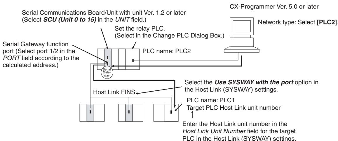
1. Register the PLC to be connected serially (using Host Link FINS) in the project gateway (e.g., PLC2).
