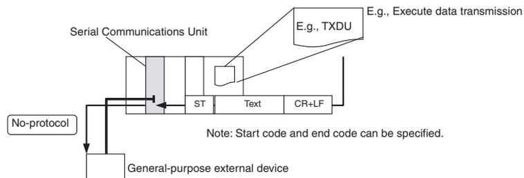
**Note** The DTXDU(262) and DRXDU(261) instructions can be used only when a CJ1W-SCU□2 Serial Communications Unit is connected to a CJ2 CPU Unit. These instructions enable faster data communications than the previous TXDU(256) and RXDU(255) instructions. Also, with the CJ1W-SCU□2, an interrupt can be generated in the CPU Unit when data is received to execute an external interrupt task.
