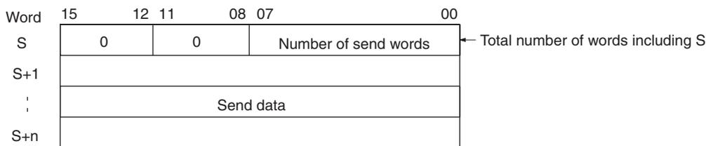
The number of send words in S+1 and the following words is stored in the rightmost 8 bits of S. The setting range is 01 to FA Hex (250 words or less). S is also included in the number of words. The data to be sent is stored in S+1 and the following words.
