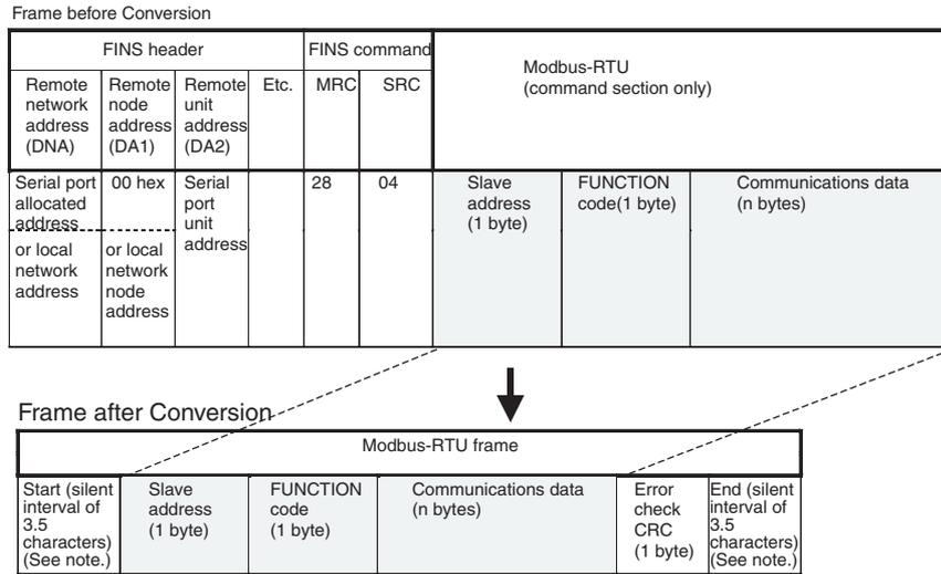
**Note** The silent interval in the Modbus-RTU frame is automatically generated by the Serial Communications Board/Unit.
