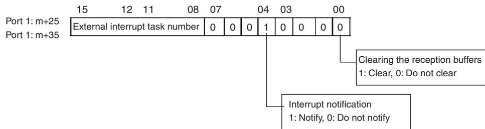
Example: The following settings are for an external interrupt task number of 5 and a Serial Communications Unit with a unit number of 0.
