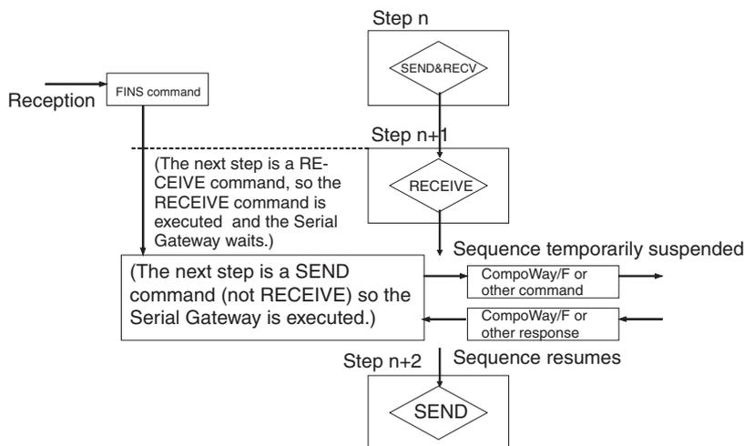
**Note** If a multiple-frame command (see note) protocol macro is sent during protocol macro execution, set the Serial Gateway mode status to prohibited (in the CIO Area). Otherwise, a FINS message converted using Serial Gateway will interrupt between steps of the executing protocol macro, and may occur in between frames of the multiple-frame command.
