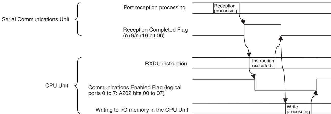
**Note** Internally, the RXDU(255) instruction uses a FINS command. Instruction processing is therefore performed in peripheral servicing. To achieve this, sometimes multiple cycles are required after the instruction is executed until the received data is stored in I/O memory.
