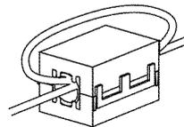
Mount the cores as close to the end of the communications cable as possible, as shown in the following illustration.
