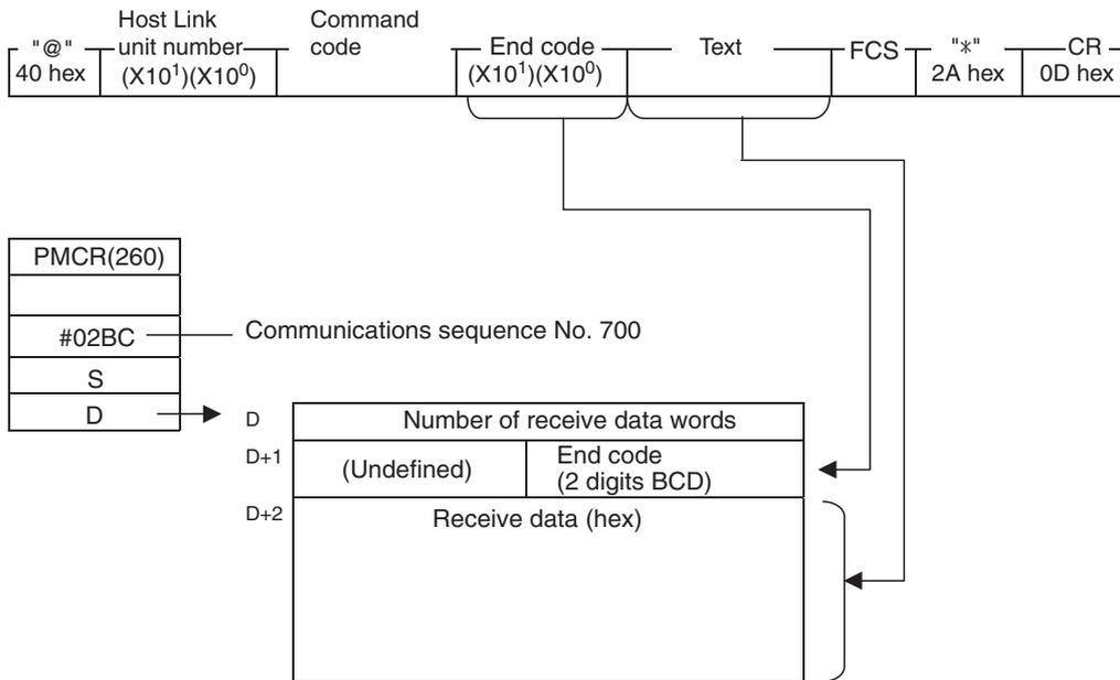
**User-specified Send/Receive Command with ASCII Conversion (Sequence No. 700 (Hex 02BC))**
