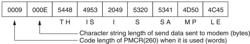
A maximum of 200 bytes (including the CR) can be received. When the received data is RETURN OK, the content stored in the receive words is as follows:
