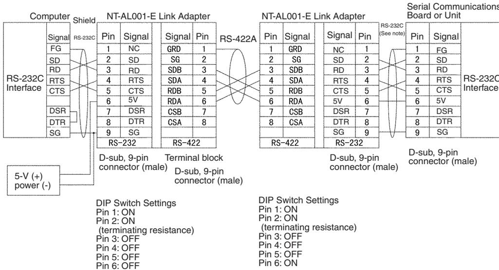
**Note** We recommend using the following NT-AL001-E Link Adapter Connecting Cables to connect to NT-AL001-E Link Adapters.
