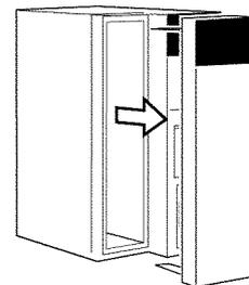
2. Install the Serial Communications Board.
