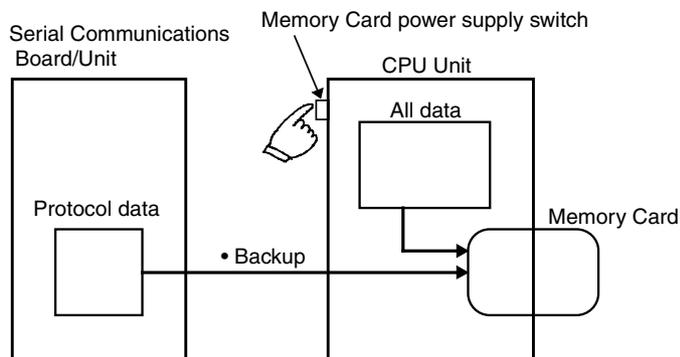
This procedure creates the Protocol Data File and writes it to the Memory Card along with the other backup files.
