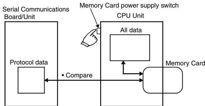
This procedure compares the protocol data in the Serial Communications Board/Unit with the data in the Protocol Data File in the CPU Unit's Memory Card.
