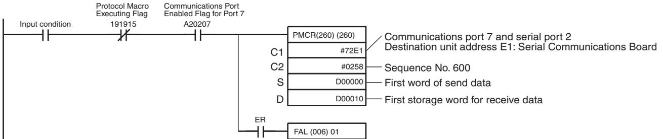
If the input condition turns ON when the Protocol Macro Executing Flag (CIO 191915 for Port 2) is OFF and the Communications Port Enabled Flag (A20207: Internal logic port, communications port 7) is ON, communications sequence No. 600 of the standard system protocol in the Serial Communications Board is called, and data is sent and received via port 2 of the Serial Communications Board.
