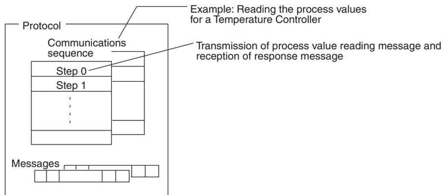
A protocol consists of processing sequences (such as reading the process value for a Temperature Controller) for a general-purpose external device. A sequence consists of a group of steps, each of which consists of a send/receive/control command, send/receive message, processing result, and a next step that depends on the processing results.
