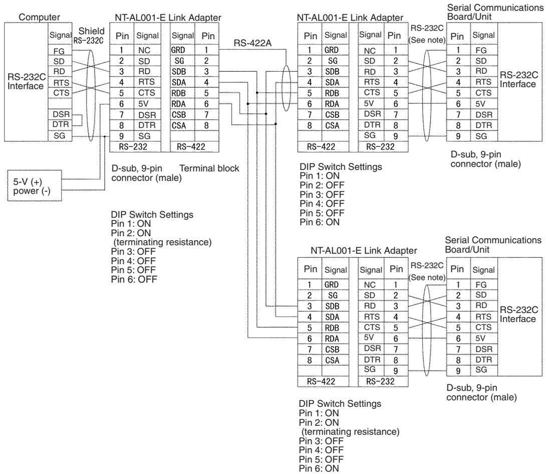
**Note** We recommend using the following NT-AL001-E Link Adapter Connecting Cables to connect to NT-AL001-E Link Adapters.
