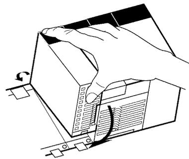
2. Insert the Unit firmly into the Backplane connector.
