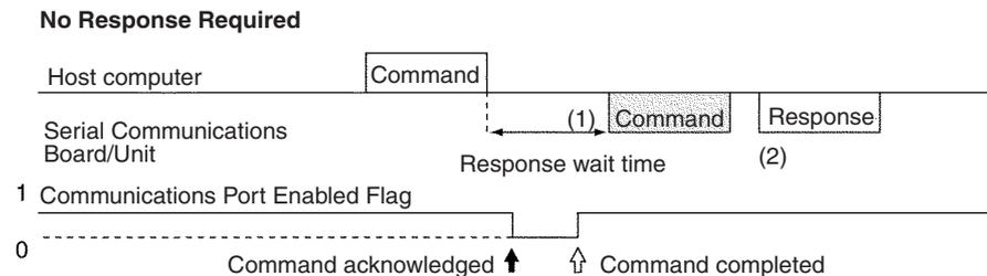
When response wait time has been set in the command format from the host computer, commands to the host computer will not be transmitted until the response time has elapsed (1). Transmission of responses to commands from the host computer will be postponed until the command transmission to the host computer has been completed (2).
