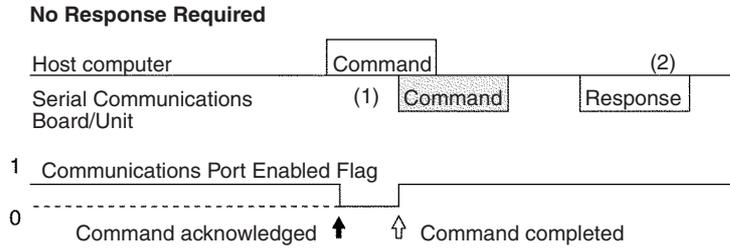
Command transmission to the host computer can start even when the port is receiving a command from the host computer (1). The transmission of a response to the command from the host computer is postponed until the transmission of the command to the host computer is completed (2).
