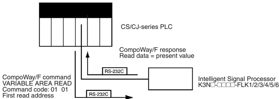
Sequence No. 600 (Send with ASCII Conversion, with Response) is used. The specified data beginning with the command code is converted ASCII and sent to the Intelligent Signal Processor with the specified node number. The response is converted to hexadecimal and stored starting at the specified word.
