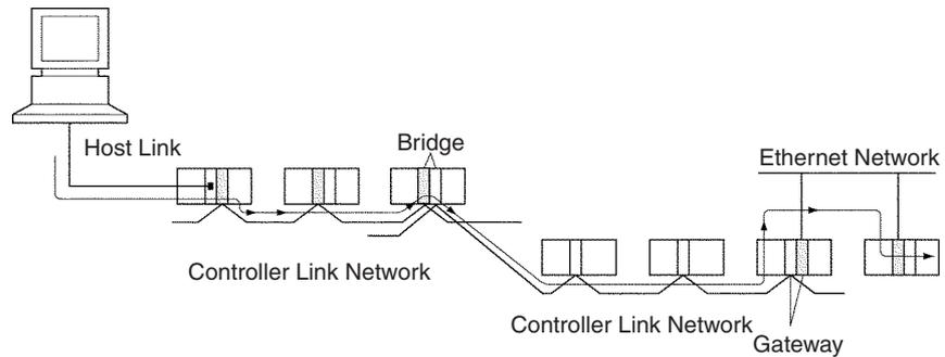
**Send FINS Commands to Computers Connected to Remote PLCs**
