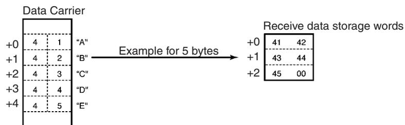
Each byte (address) in the Data Carrier contains the code for one ASCII character.
