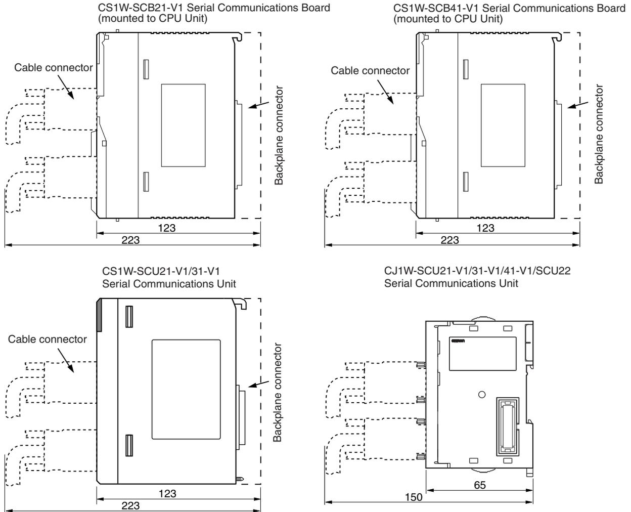
**Note** The mounting heights shown above are applicable when the attached connectors, connector covers, and recommended cables are used. The mounting height may differ when other connectors, connector covers, and cables are used. Determine the mounting height, taking into account the connectors, connector covers, and the minimum bending radius of the cables.
