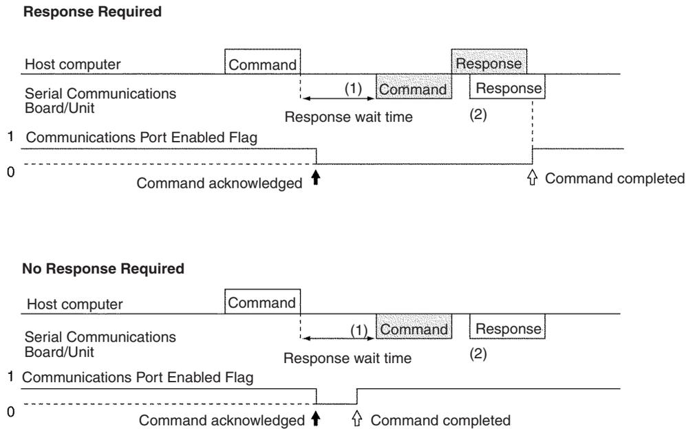
When response wait time has been set in the command format from the host computer, commands to the host computer will not be transmitted until the response time has elapsed (1). Transmission of responses to commands from the host computer will be postponed until the command transmission to the host computer has been completed (2).
