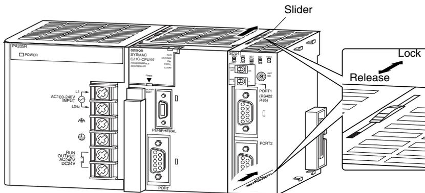
**Note** If the sliders are not locked properly, the Serial Communications Units may not function correctly.
