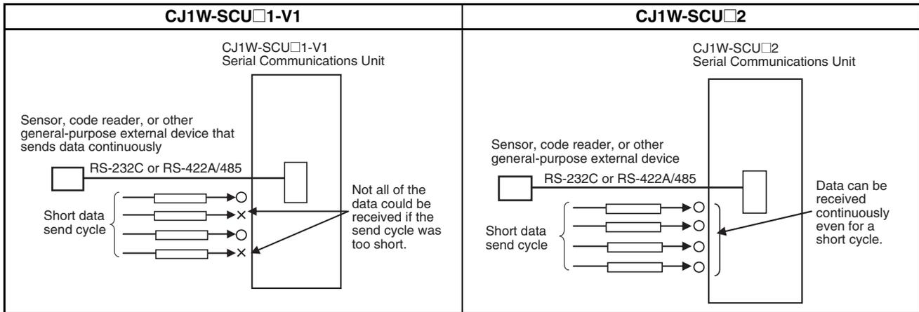
The following table lists the cycle times for which data can be received continuously.
