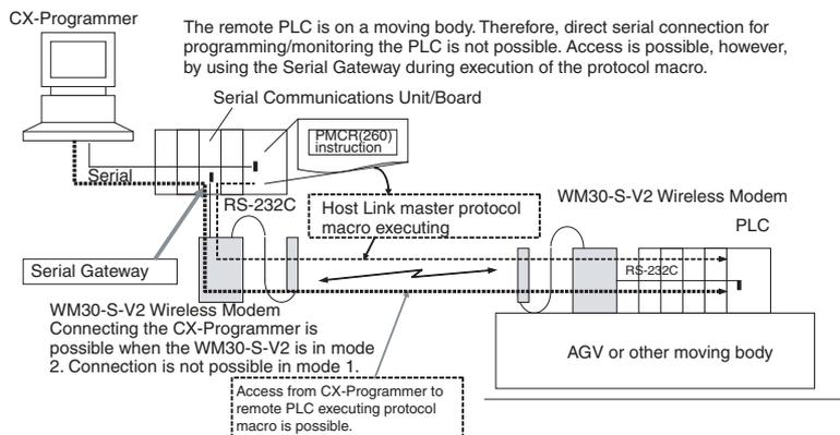
**Note** If the Serial Gateway Prohibit Switch allocated in the CIO Area is OFF, the Serial Gateway is enabled whether protocol macros are being executed or not. During execution of protocol macros, however, the Serial Gateway is processed using interrupts between steps in the communications sequence.
