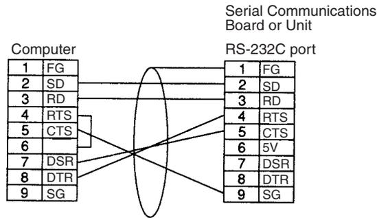
**Connecting a Host Computer with NT-AL001-E Converting Link Adapters**
