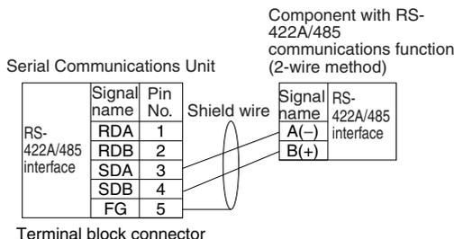
**Note** Be sure to connect terminating resistance of between 100 and 125 Ω (1/2 W) to the terminals of the remote devices at either end of the RS-422A/485 transmission path. (Set the terminating resistance on the Board/Unit by turning ON/OFF the Terminating Resistance Switch.)
