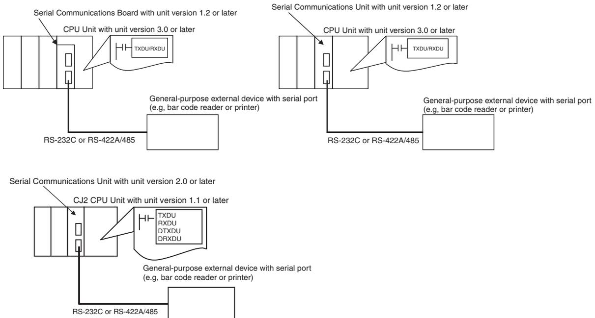
Addition of a start code at the beginning of the data, and end code at the end of the data (or specifying the number of receive data bytes) is possible before sending/receiving. The RS and CS control signals can also be controlled.
