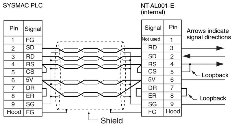
**Note** The XW2Z-□□0T-1 Connecting Cable for the NT-AL001-E Link Adapter uses special wiring for the DS and RS signals. Do not use these Cables with other devices. If these Cables are connected to other devices, the devices may be damaged.
