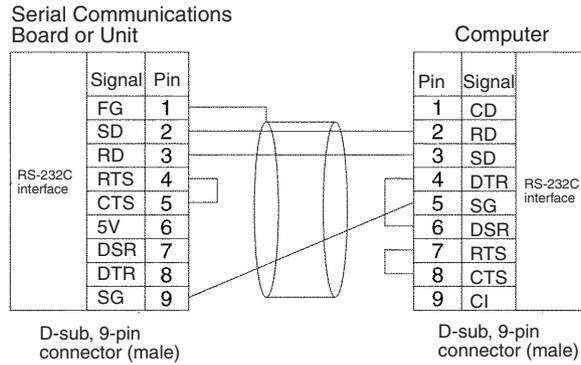
Using NT-AL001-E Converting Link Adapters
