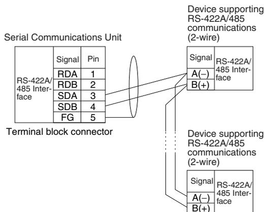
**Note** Be sure to connect terminating resistance of between 100 and 125 Ω (1/2 W) to the terminals of the remote devices at either end of the RS-422A/485 transmission path. (Set the terminating resistance on the Board/Unit by turning ON/OFF the Terminating Resistance Switch.)
