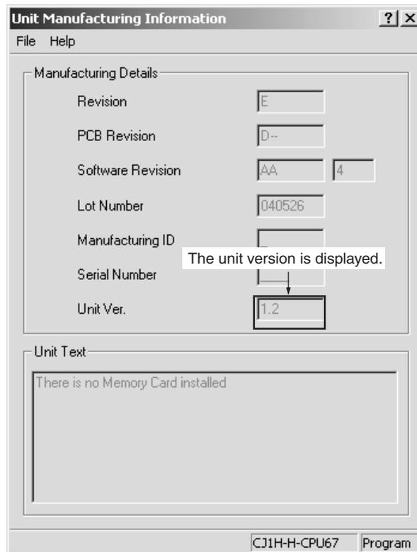
Example: In this Unit Manufacturing Information Dialog Box, unit version 1.3 is displayed. Use this dialog box to confirm the unit version of the Serial Communications Unit that is connected online.
