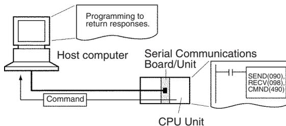
SEND(090) can be used to send data from the PLC to a host computer. If the input condition turns ON when the Communications Port Enabled Flag is ON, 10 words of data from CIO 0100 to CIO 0109 will be sent to the host computer connected to port 1 on the Serial Communications Unit with network address 0, node address 0, and unit address 10 Hex.
