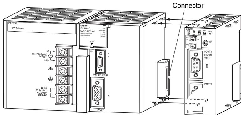
2. Slide the sliders on the top and bottom of the Unit until they lock the Units together.
