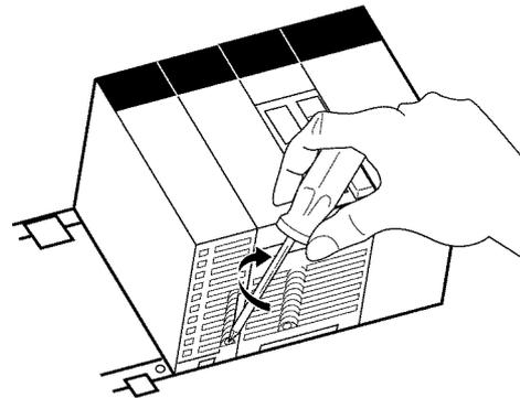
**Note** Tighten the screw to a torque of 0.4 N-m.
