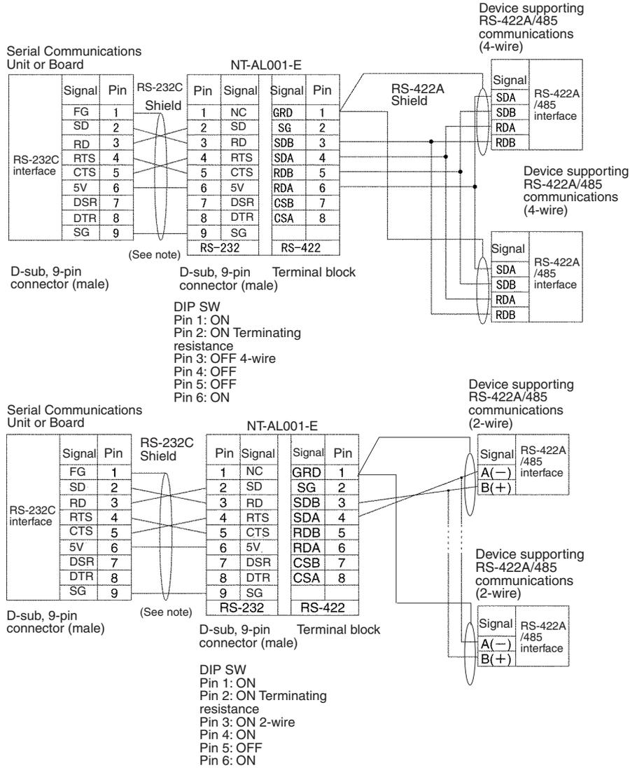
**Note** We recommend using the following NT-AL001-E Link Adapter Connecting Cables to connect to NT-AL001-E Link Adapters.
