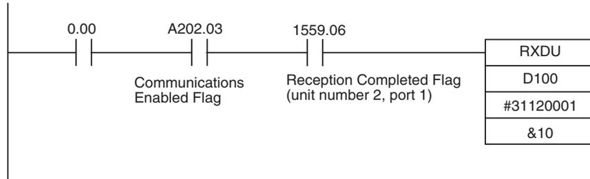
**Note** Use an AND between an NO condition of the Communications Enabled Flag (A202.03) and an NC condition of the Reception Completed Flag (n+9/n+19 bit 06) when executing RXDU(255) for a Unit.
