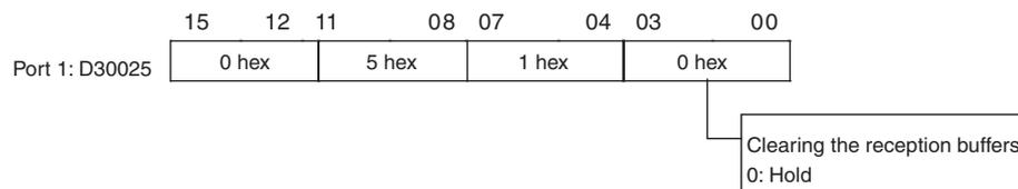
The above words allocated in the DM Area can be set from the **Unit Setup** for the Serial Communications Unit in the I/O Table Window.
