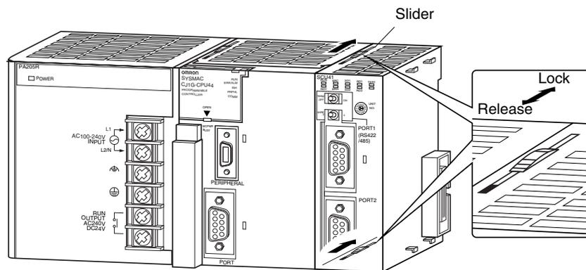
**Note** If the sliders are not locked properly, the Serial Communications Units may not function correctly.
