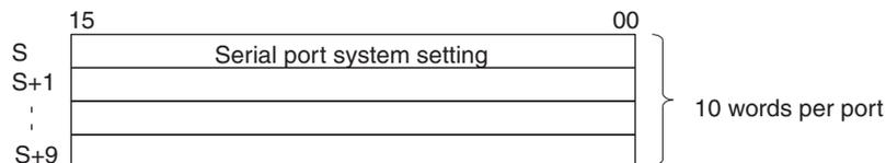
When the STUP(237) instruction is executed, the CPU Unit changes the contents of the relevant DM Area in the Unit, then automatically turns ON the Port Settings Change Bit (words A620 to A635) in the Auxiliary Area.
