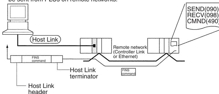
Unit version 1.2 or later supports the 1:1 Host Link protocol for C200H, C1000H, and C2000H CPU Units, which enables the use of host programs for 1:1 Host Links created for these PLCs. A Host Link-compatible device selection function is also provided for complete compatibility with the C-series Host Link and CVM1/CV-series Host Link.
