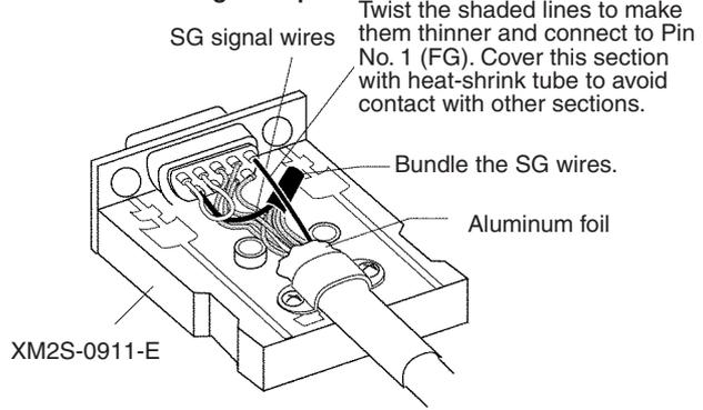
**Note** The Hood (FG) is internally connected to the ground terminal (GR) on the Power Supply Unit via the CPU Rack or Expansion Rack. Therefore, FG is grounded by grounding the ground terminal (GR) on the Power Supply Unit. Although there is conductivity between the Hood (FG) and pin 1 (FG), connect the Hood (FG) to the shield because the Hood (FG) has smaller contact resistance with the shield than pin 1 (FG), and thus provides better noise resistance.
