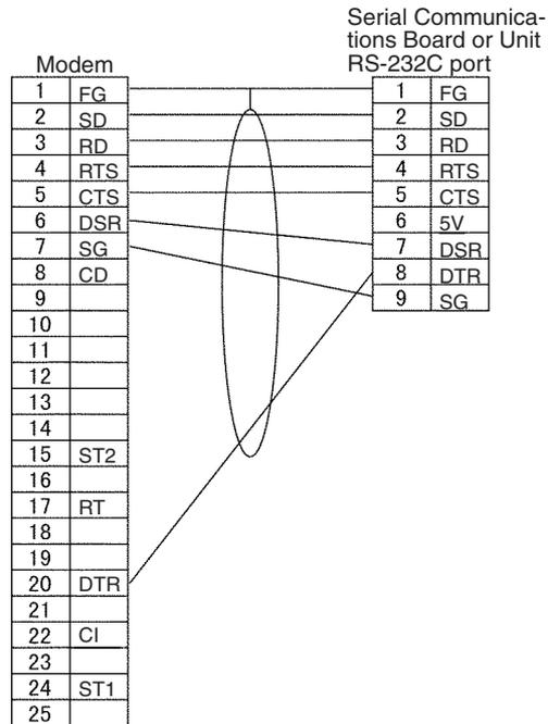
1:N Connections Using RS-232C Ports
