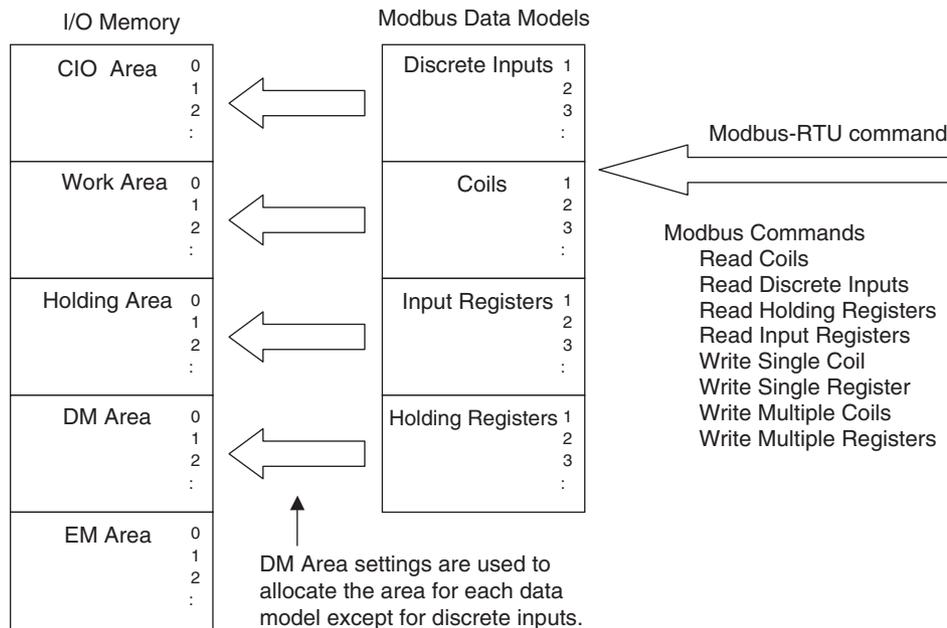
Refer to 9-2 Setup Area Allocations (Modbus-RTU Slave Mode) for the DM Area settings to allocate areas. Refer to 9-3-4 Command and Response Details for details on Modbus-RTU commands.
