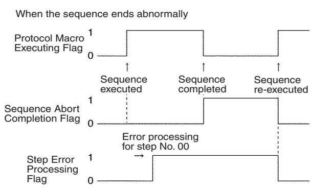
**Note** The Step Error Processing Flag is used to see whether error processing has been executed for an individual step in a sequence, and not for the overall steps. Therefore, as shown in Example 2 above, after executing error processing during a sequence (step No. 00), the flag will remain ON, even if the next step ends normally. Care is therefore required because it is not always possible to use this flag to determine whether the overall sequence has ended abnormally.
