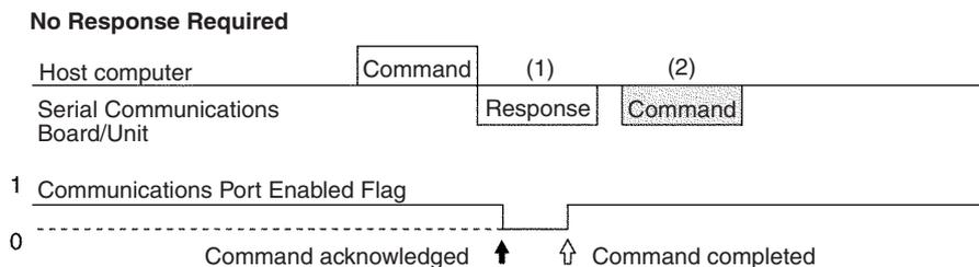
At (1) in the diagram, the response to a command sent from the host computer is being transmitted from the port. In this case, the command transmission to the host computer is postponed until the response transmission is completed (2).
