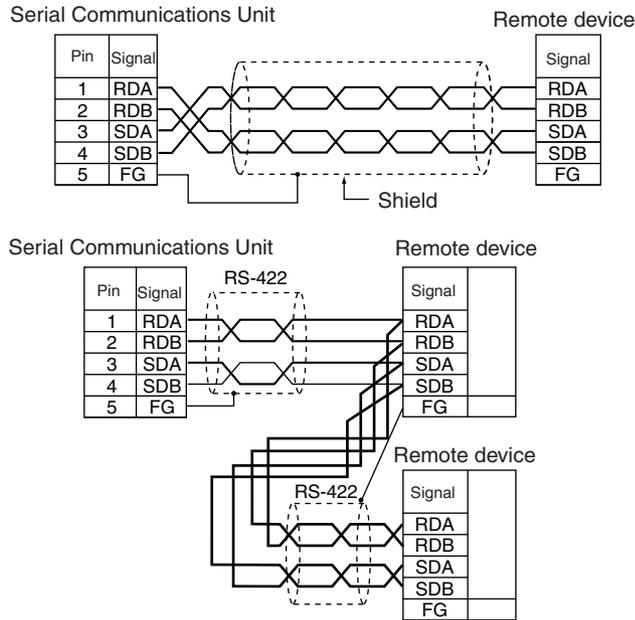
**Note** The Hood (FG) is internally connected to the ground terminal (GR) on the Power Supply Unit via the CPU Rack or Expansion Rack. Therefore, FG is grounded by grounding the ground terminal (GR) on the Power Supply Unit.
