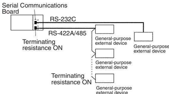
Also perform other required processing, such as setting switches on the external device(s).
