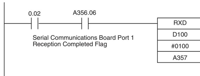
**Note** Use an AND of an NO condition of the Reception Completed Flag (A356 bit 06/14) in the input conditions when executing the RXD(235) instruction for a Board.
