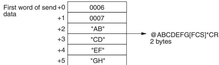
2. At reception, data excluding the header code “@” at the beginning of the receive data and the FCS and terminator “\*”CR at the end of the data is stored in the receive data storage words.
