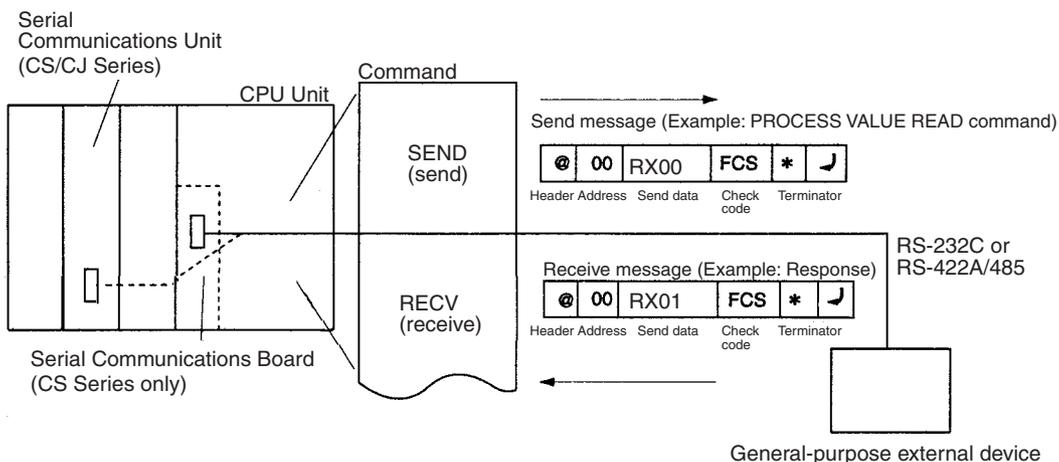
Depending on the response received, the user can either choose to resend the same send message (retry processing), or to perform the next process (for example, read the process value for a Temperature Controller with a different address).
