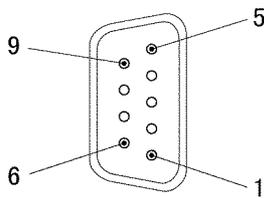
This layout applies to the following ports: ports 1 and 2 of the CS1W-SCB21-V1/SCU21-V1, ports 1 and 2 of the CJ1W-SCU21-V1/SCU22, port 1 of the CS1W-SCB41-V1, and port 2 of the CJ1W-SCU41-V1/SCU-42.
