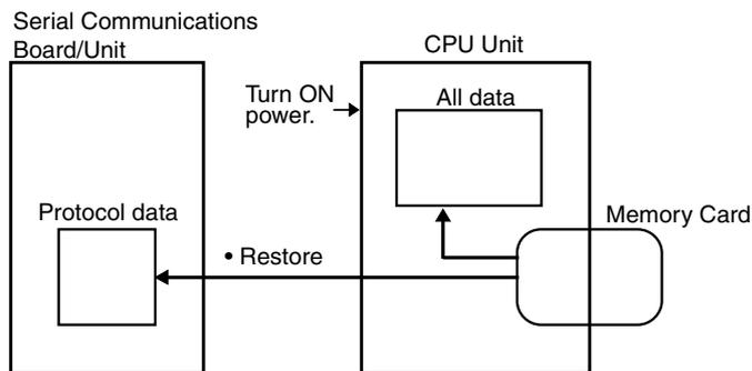
This procedure reads the Serial Communications Board/Unit's Protocol Data File from the Memory Card and sets that data in the Serial Communications Board/Unit.
