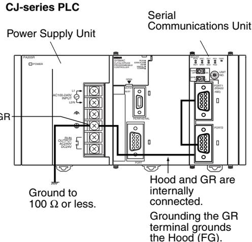
**3-4-3 Wiring Connectors for the CS1W-SCB□1-V1, CS1W-SCU□1-V1, CJ1W-SCU□1-V1, or CJ1W-SCU22/42 (RS-232C Connector Only)**
