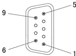
This layout applies to the following ports: port 2 of the CS1W-SCB41-V1, ports 1 and 2 of the CS1W-SCU31-V1, ports 1 and 2 of the CJ1W-SCU31-V1, and port 1 of the CJ1W-SCU41-V1.
