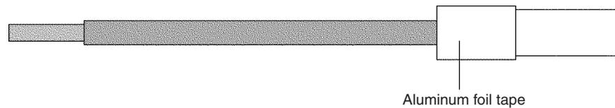
**Shield Not Connected to Hood (FG)**
