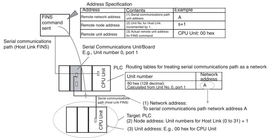
6-7-3 Using a non-PLC Component as the Target
