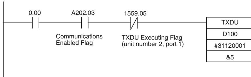
**Note** Use an AND between an NO condition of the Communications Enabled Flag (A202.03) and an NC condition of the TXDU Executing Flag (n+9/n+19 bit 05) when executing TXDU(256) for a Unit.
