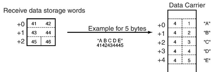
Each byte (address) in the Data Carrier contains the code for one ASCII character.
