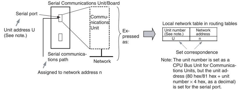
The Routing Table Setting Tool in the CX-Integrator or CX-Net is used to set the relationship between the serial port's unit address and the allocated network address in the local network tables of the routing tables. These settings are then transferred to the CPU Unit to which the Serial Communications Unit/Board is mounted.
