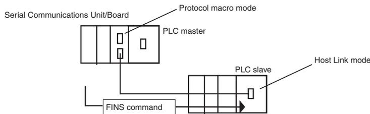
**Note** The remote destination network address (DNA) specifies the local network address (00 hex), the remote destination node address (DA1) specifies the local node (00 hex), and the remote destination unit address (DA2) specifies the CPU Unit in the PLC Slave (00 hex).
