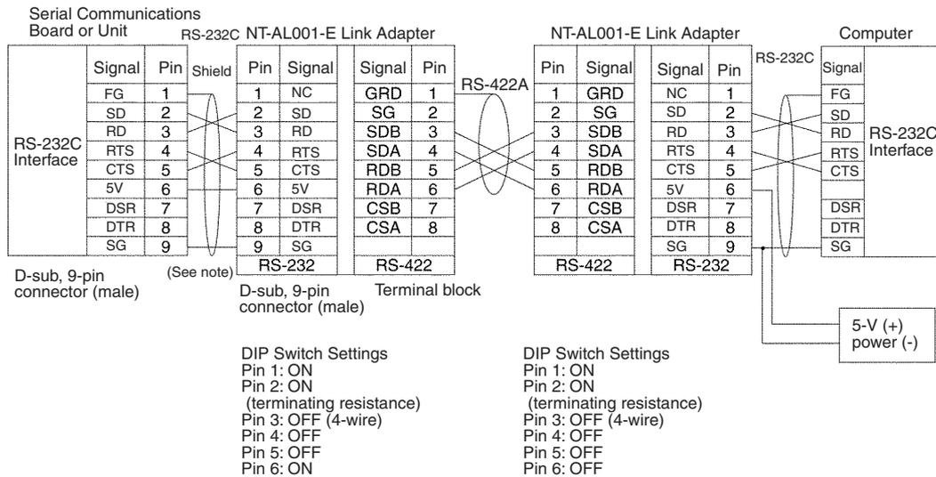
**Note** We recommend using the following NT-AL001-E Link Adapter Connecting Cables to connect to NT-AL001-E Link Adapters.
