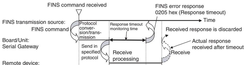
**Note** If a Serial Gateway response timeout occurs, CIO word n+8/n+18, bit 05 (Serial Gateway Send Start Timeout or Serial Gateway Response Timeout)
