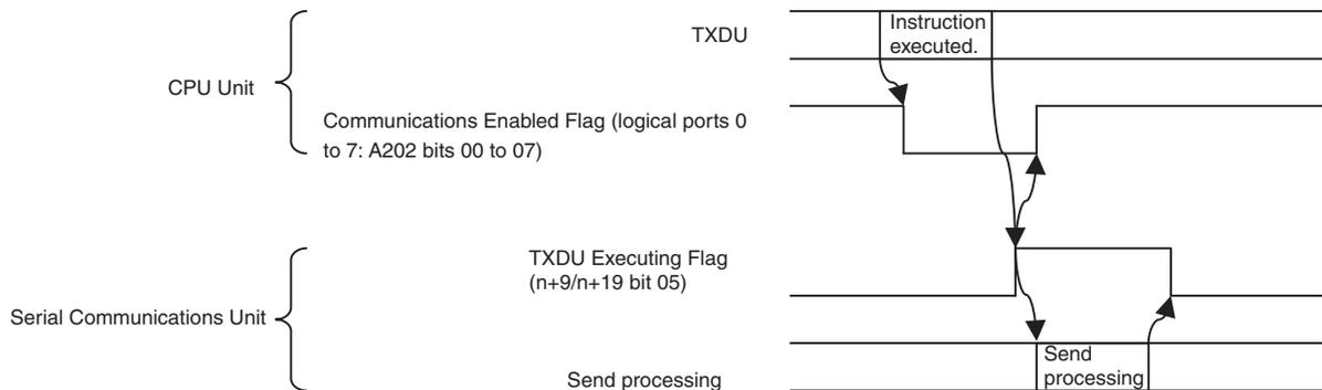
**Note** Internally, the TXDU(256) instruction uses a FINS command. Instruction processing is therefore performed in peripheral servicing. To achieve this, sometimes multiple cycles are required after the instruction is executed to process the send.
