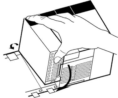
2. Make sure that the connector on the back of the Unit is properly inserted into the connector in the Backplane.
