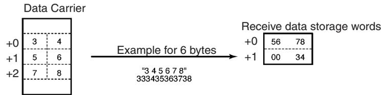
Each byte (address) in the Data Carrier contains 2 digits.
