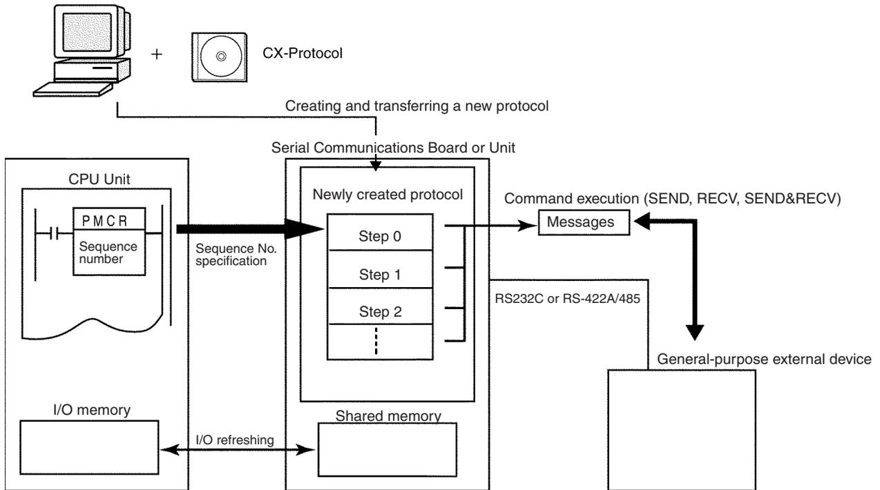
In this manual, the protocol structure is explained in simple terms, and examples are given of the use of the PMCR(260) instruction when controlling
