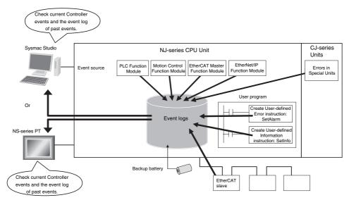
To use an NS-series PT to check events, connect the PT to the built-in EtherNet/IP port on the CPU Unit.
