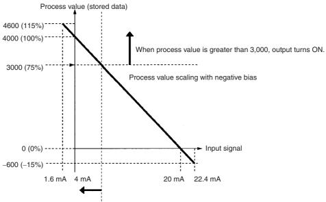
When input signal is less than 8 mA, output turns ON.
