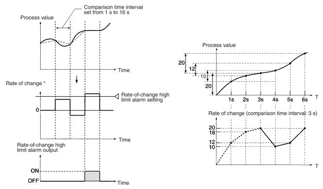
\* The rate-of-change value is derived by taking the difference each second between the process value at that time and the process value before the comparison time interval, rather than the difference calculated at each comparison time interval. This allows even a very small process value change to be detected.
