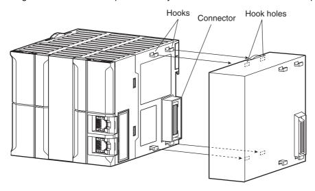
Move the sliders on the top and bottom of the Unit to the lock position to secure the Units. The sliders should click into place.
