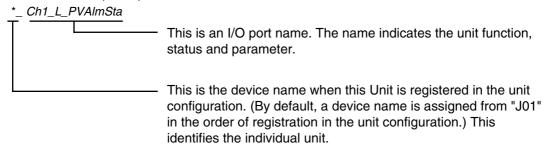
In the explanations from here on, the device name automatically created is used as the device variable for CJ-series Unit, for example \* Ch1 L PVAlmSta.
