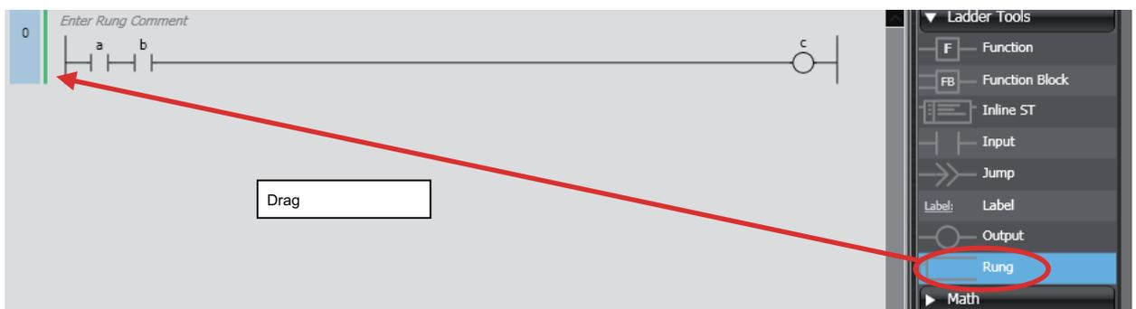
**Method (2) Select the start of a rung and press the R Key. (Press the Shift + R Keys to insert a rung above the selected rung.)**
