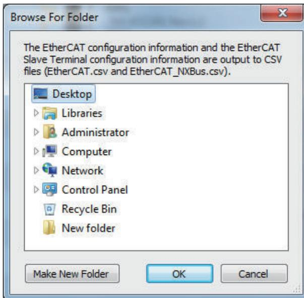
CSV files (comma delimited) that contain the EtherCAT network configuration information and the EtherCAT Slave Terminal configuration information are saved in the selected folder.
