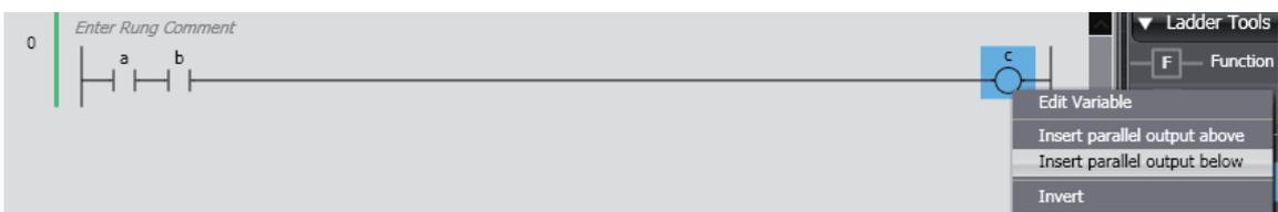
The output is inserted in an OR structure.
