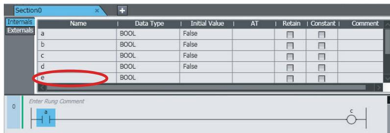
In this case, any variables assigned to the input are not deleted from the local variable table or global variable table.
