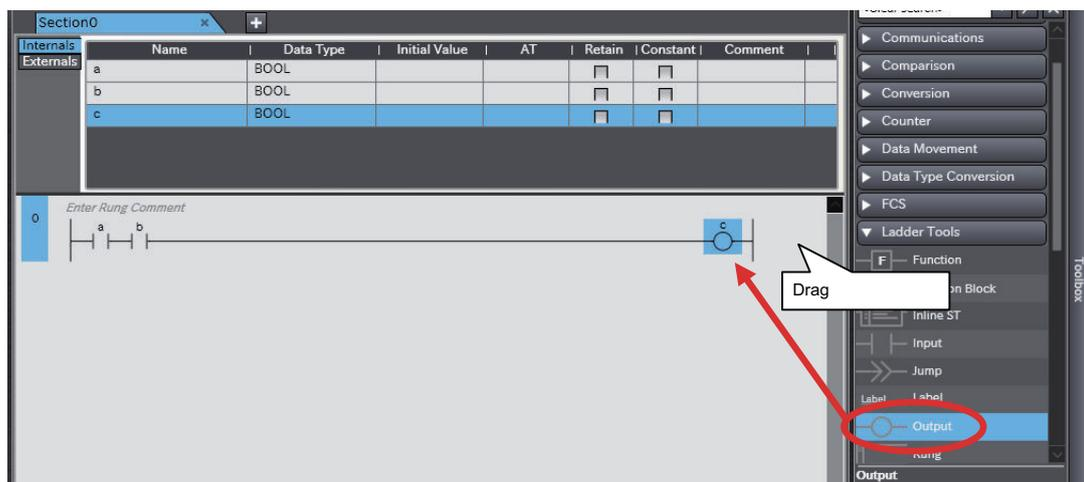
The output is inserted.
