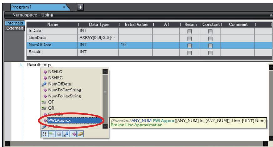
The selected function or function block instance is displayed. When you enter a *left parenthesis*, a description of the parameters is displayed.
