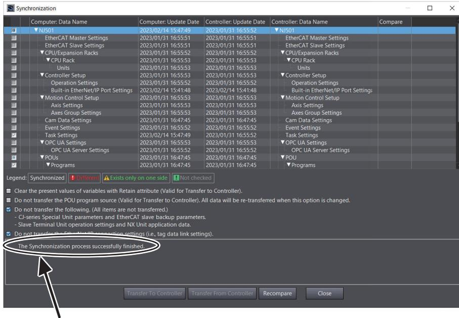
This is displayed if the synchronization process is completed successfully.
