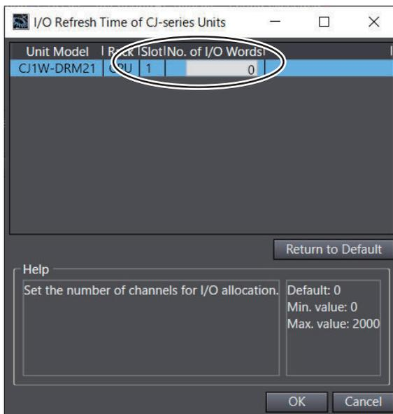
The size of the expansion areas is used to calculate the I/O refresh time for the specific CJ-series Special Units.
