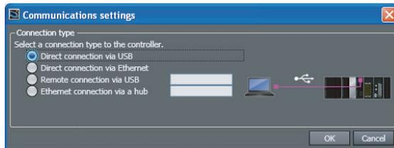
The IP address that is set in the Communications Setup Dialog Box is displayed to the right of the remote connection methods.
