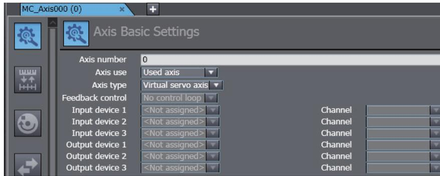
The Axis Parameter Settings tab page is displayed in the Edit Pane. The *basic parameters* are displayed on the initial display.
