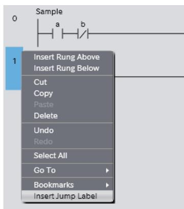
Or, drag a **Label** under **Ladder Tools** in the **Toolbox** to the beginning of the rung. A jump label entry field is inserted.
