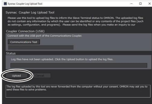
The Slave Terminal log is uploaded from the Slave Terminal and the directory where the log files were saved is displayed in the **Status** area.
