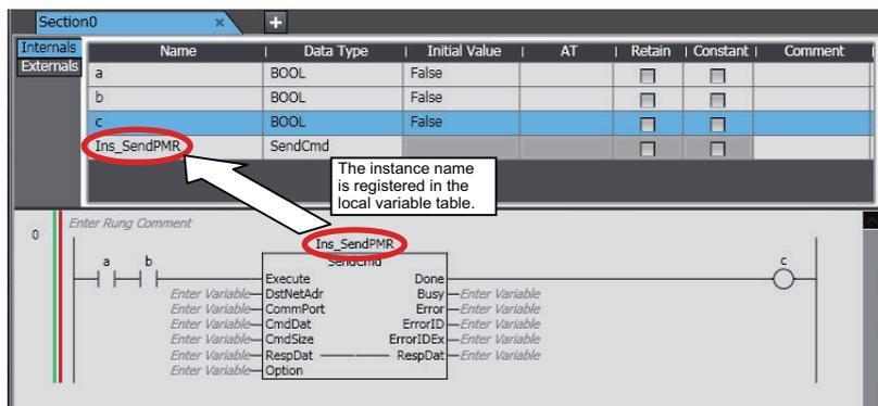
This completes the insertion of the function block. If you entered a new instance name, it is registered in the local variable table.
