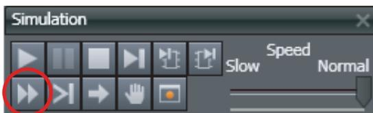
The cursor moves to the next execution step in the ST Editor after a fixed period of time (1 second). The time required to move to the next step depends on the program.
