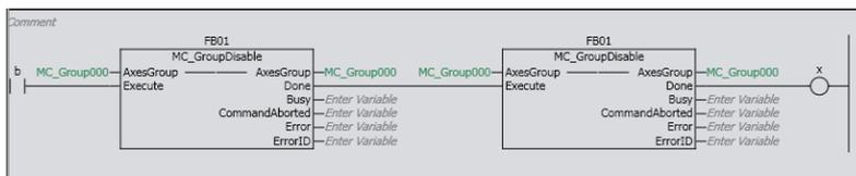
If a circuit part is selected, the function block instance is pasted under that circuit part.
