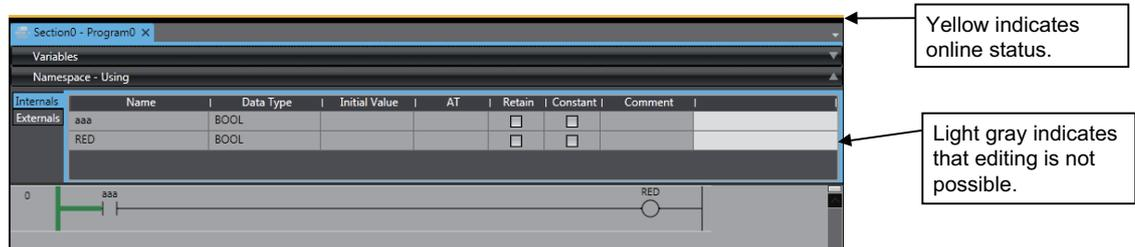
The TRUE/FALSE status of the connecting lines is displayed while the task is executed in RUN mode.
