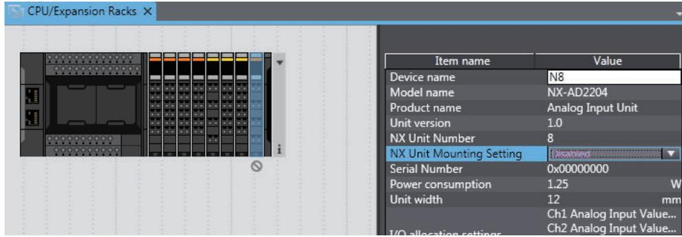
Change the setting to **Enabled** in the Unit setting item list to enable the Unit again.
