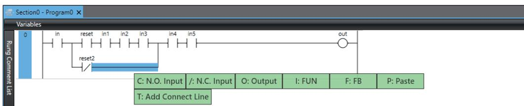
The connecting line movement guide appears when you perform the following operation.
