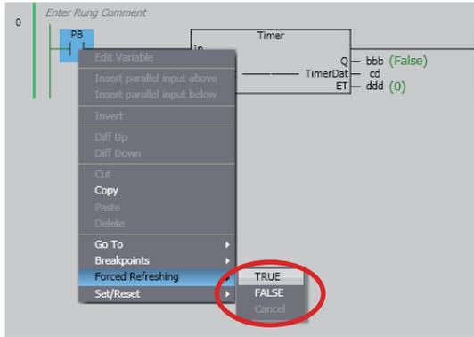
The input or output in the Ladder Editor changes to TRUE or FALSE and the execution condition changes accordingly.
