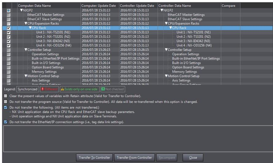
The CPU Rack configuration information is downloaded from the Sysmac Studio to the Controller.
