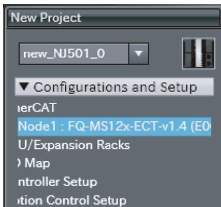
The Setup Tab Page for the **FQ-MS12x-ECT...** is displayed for the Edit Pane. Make all of the required setting. Refer to the *FQ-M-series Specialized Vision Sensor for Positioning User's Manual (Cat. No. Z314)* for the setup procedures.
