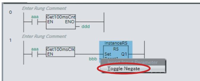
The input for the selected parameter is inverted.
