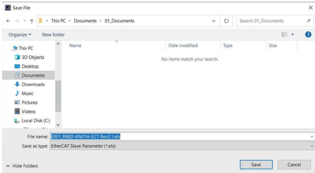
An EtherCAT slave parameter file with an .ets extension is saved.
