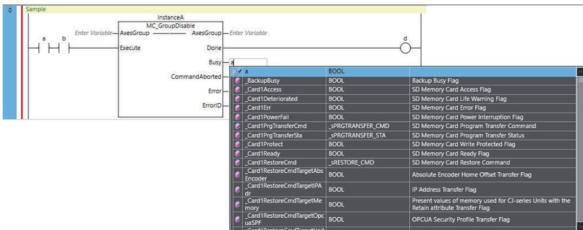
All variables with the correct data type are displayed in the list. The selected variable is entered into the function block.
