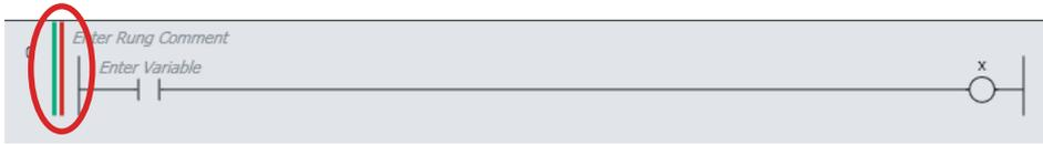
Place the mouse over the red line to view information on the rung error.
