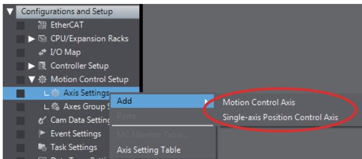
The axis *MC\_Axis000(0)* is added under **Axis Settings**.
