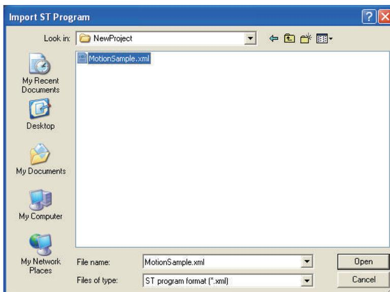
The data is imported and the programs, functions, function blocks, data types, and global variables in the XML file are added to the project.
