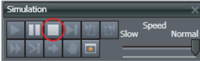
The connection to the Simulator is broken and the Simulator is exited.
