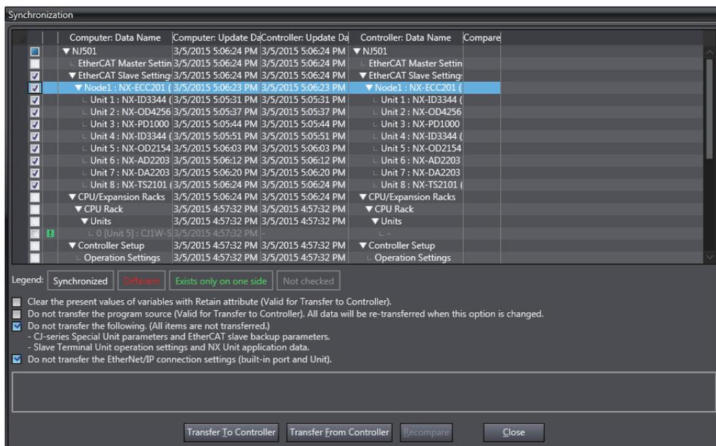
The Slave Terminal configuration information is downloaded from the Sysmac Studio to the Controller.
