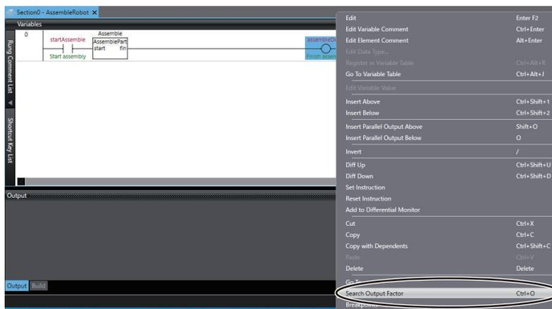
The ladder diagram rung that includes the target of the output factor search is displayed on the Search Output Factor Tab Page.
