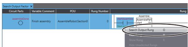
The target output rung is displayed under the selected circuit part.
