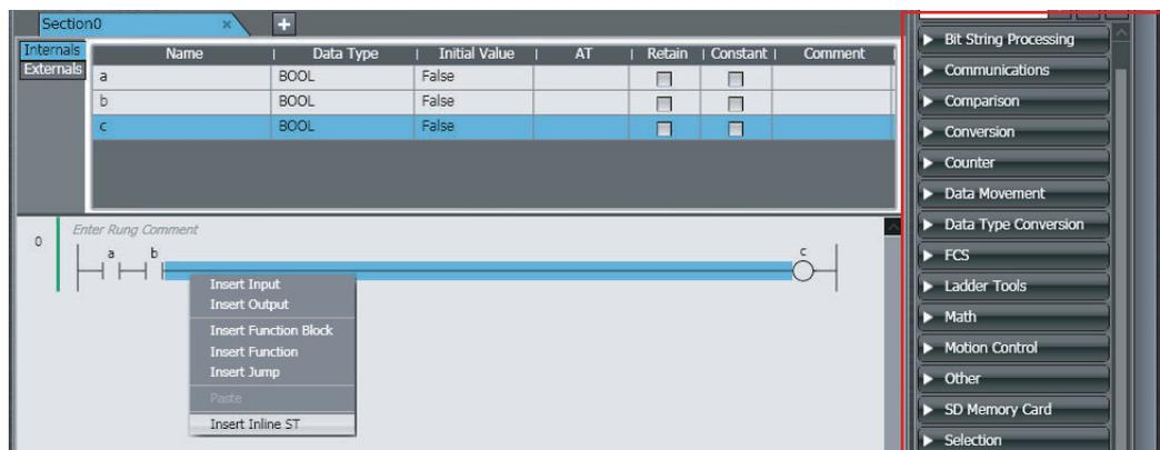
An inline ST box is inserted.
