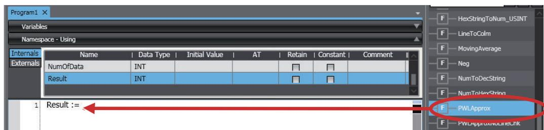
The function or function block is inserted with temporary variables.
