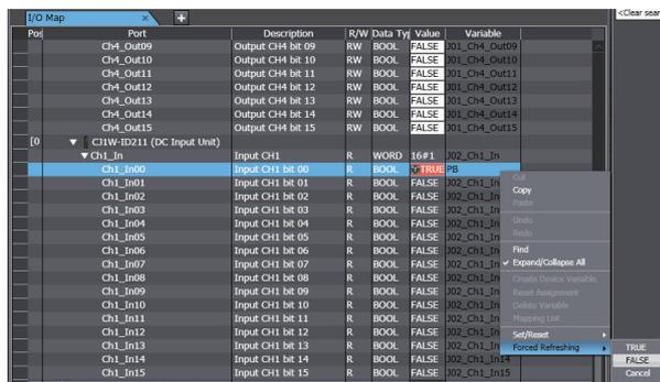
After you force the BOOL device variable to TRUE or FALSE, the value in the **Value** column in the I/O Map changes to TRUE or FALSE to reflect that change.
