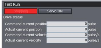
The Servo turns ON and motor control is enabled.
