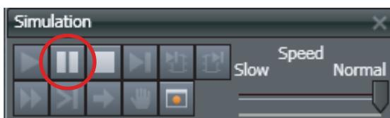
The cursor stops moving. Execution of the program is paused, but the Simulator does not close.
