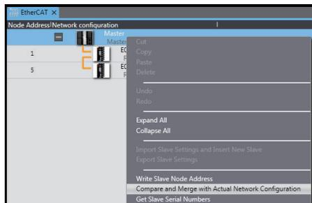
The actual network configuration is read and compared with the network configuration on the Sysmac Studio. The results are displayed in the **Compare and Merge with Actual Network Configuration** Dialog Box.
