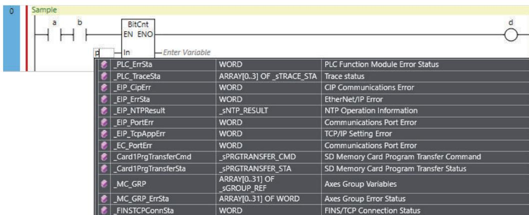
All variables with the correct data type are displayed in the list. The selected variable is entered into the function.
