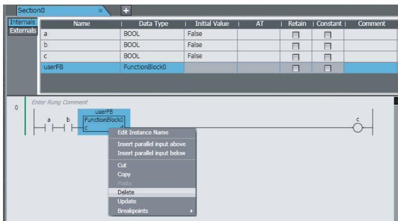
The selected function block instance is deleted. However, the variables used for parameters are not deleted.
