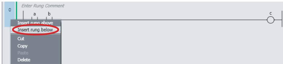
A rung is inserted above or below the selected rung.
