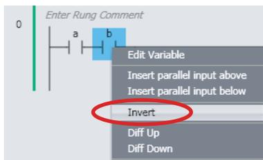
The N.O./N.C. state of the input or output is reversed.
