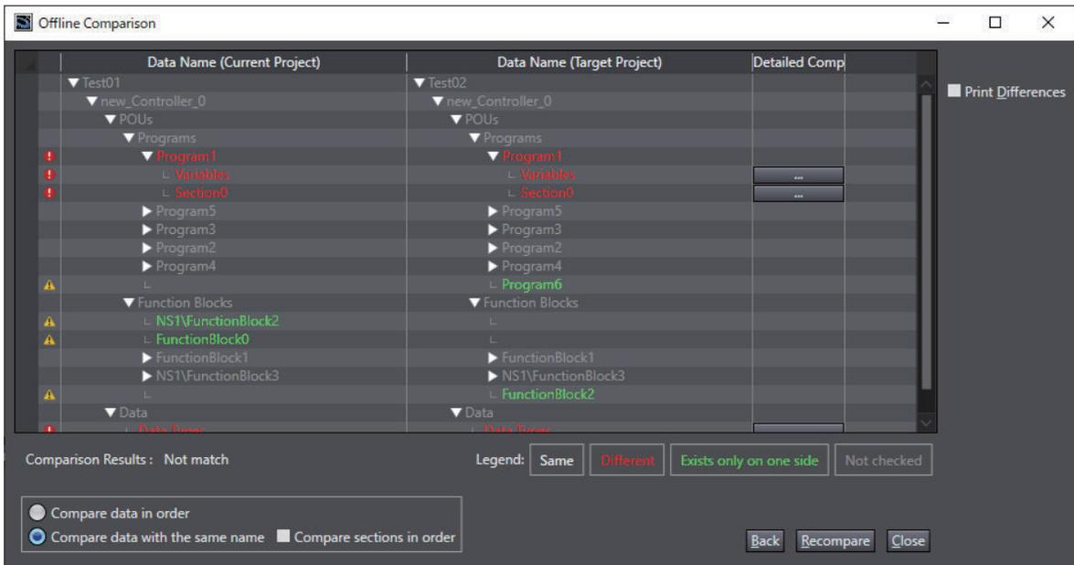
The units for comparison that are shown in the Offline Comparison Window are listed in the following table.
