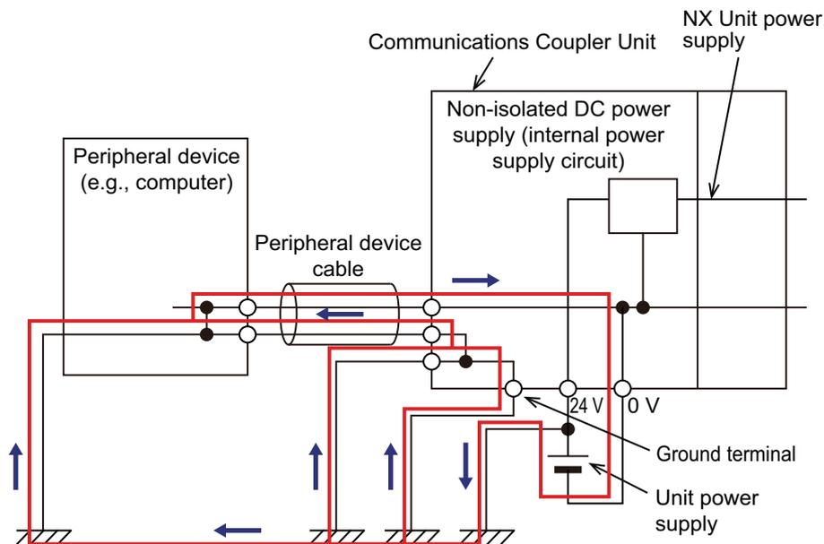
Be sure that all terminal screws and cable connector screws are tightened to the torque specified in the relevant manuals. The loose screws may result in fire or malfunction.
