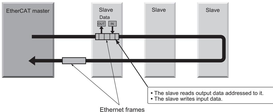
The data exchanges that are cyclically performed between the EtherCAT master and EtherCAT slaves use EtherCAT datagrams that are stored directly in the Ethernet frames.
