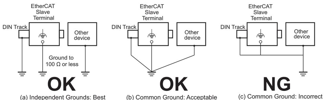
If the DIN Track is made of steel and the surface is not treated to produce an insulating material, you can omit grounding the functional ground terminal on any Unit that has one, as shown in the following figures.
