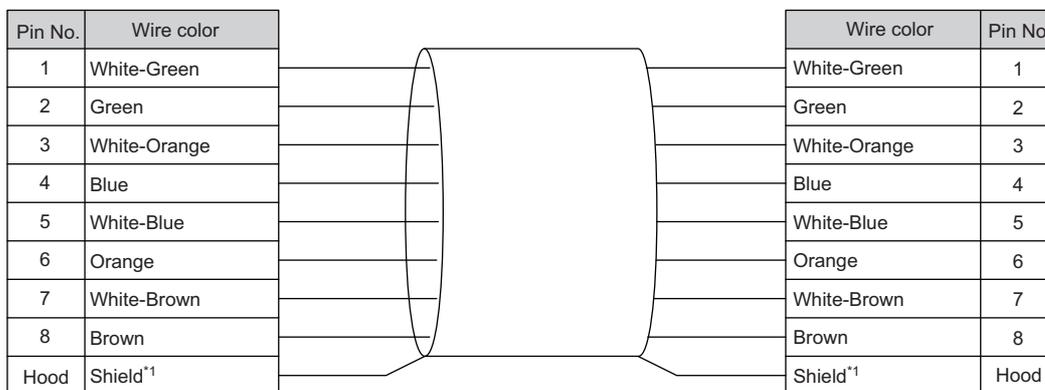
\*1. Connect the cable shield wire to the connector hood at both ends of the cable.
