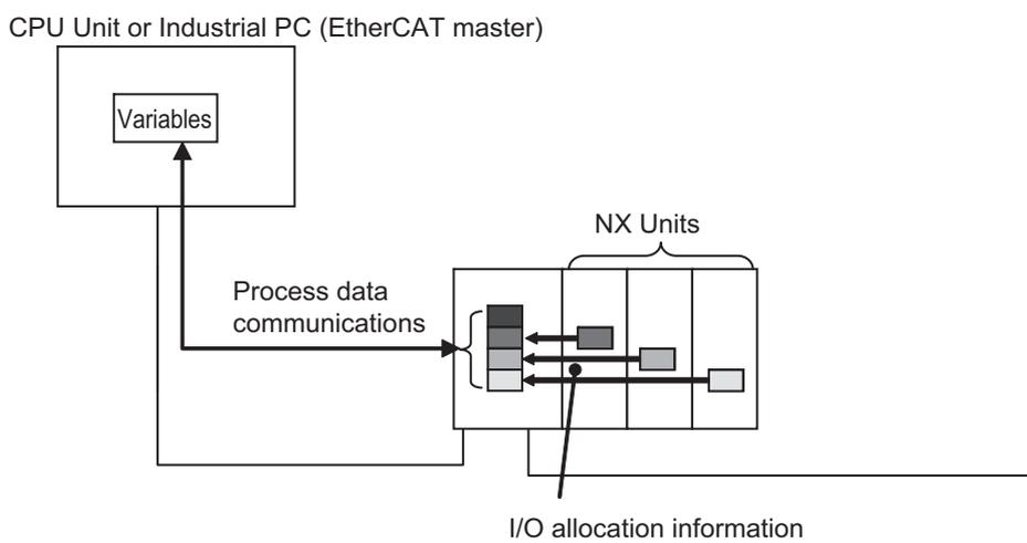
The EtherCAT Coupler Unit and the NX Units contain default values for the I/O allocation information. These default values are sufficient for a standard exchange of I/O data. Change the settings as necessary.
