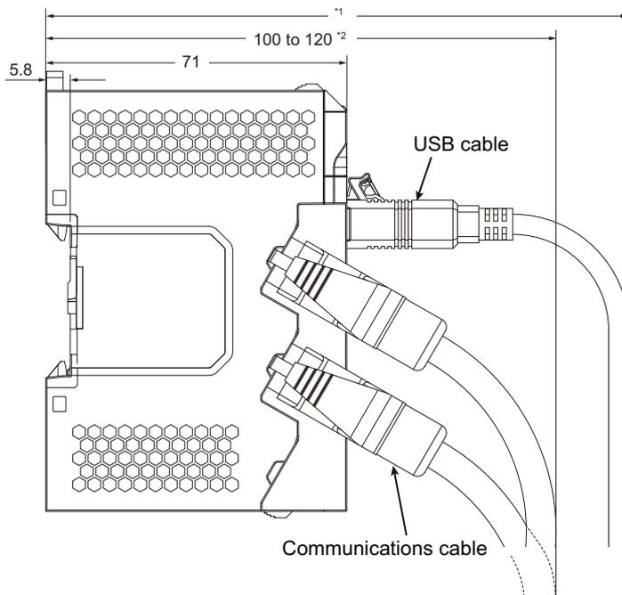
\*1. This dimension depends on the specifications of the commercially available USB certified cable. Check the specifications of the USB cable that is used.
