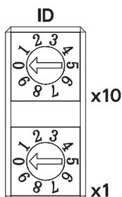
Refer to 4-3-3 *Setting the Node Address* on page 4-12 for information on setting the node address by combining the rotary switches and pin 4 of the DIP switch that is described below.
