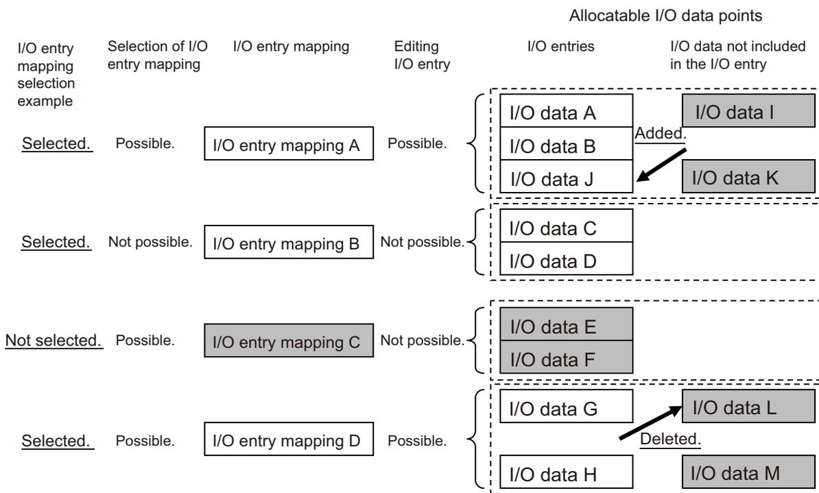
\*The shaded I/O data is not exchanged with process data communications.
