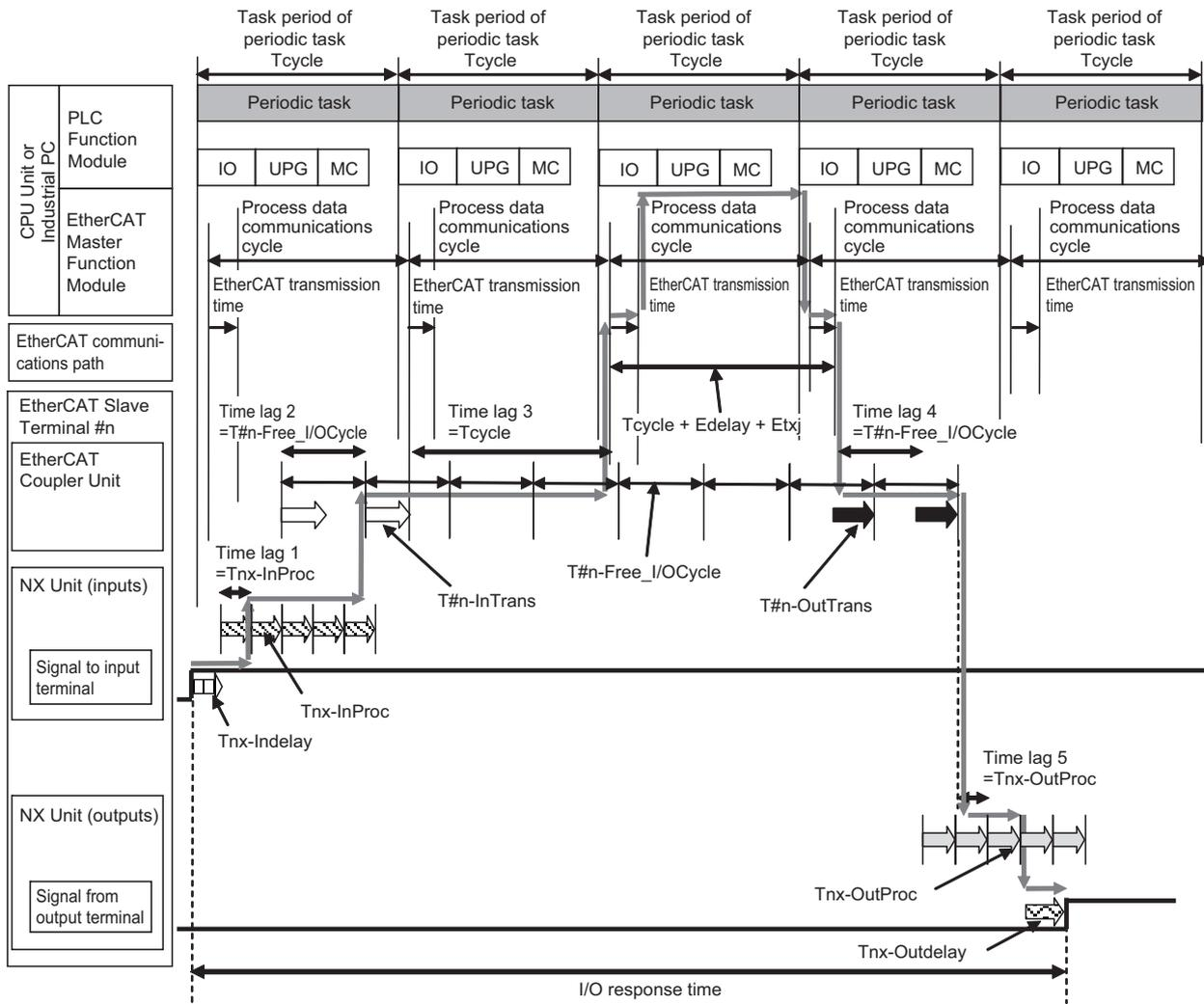
The maximum and minimum values of the I/O response time are calculated as shown below. The minimum value occurs when the time lags that are shown in the above figure do not occur.
