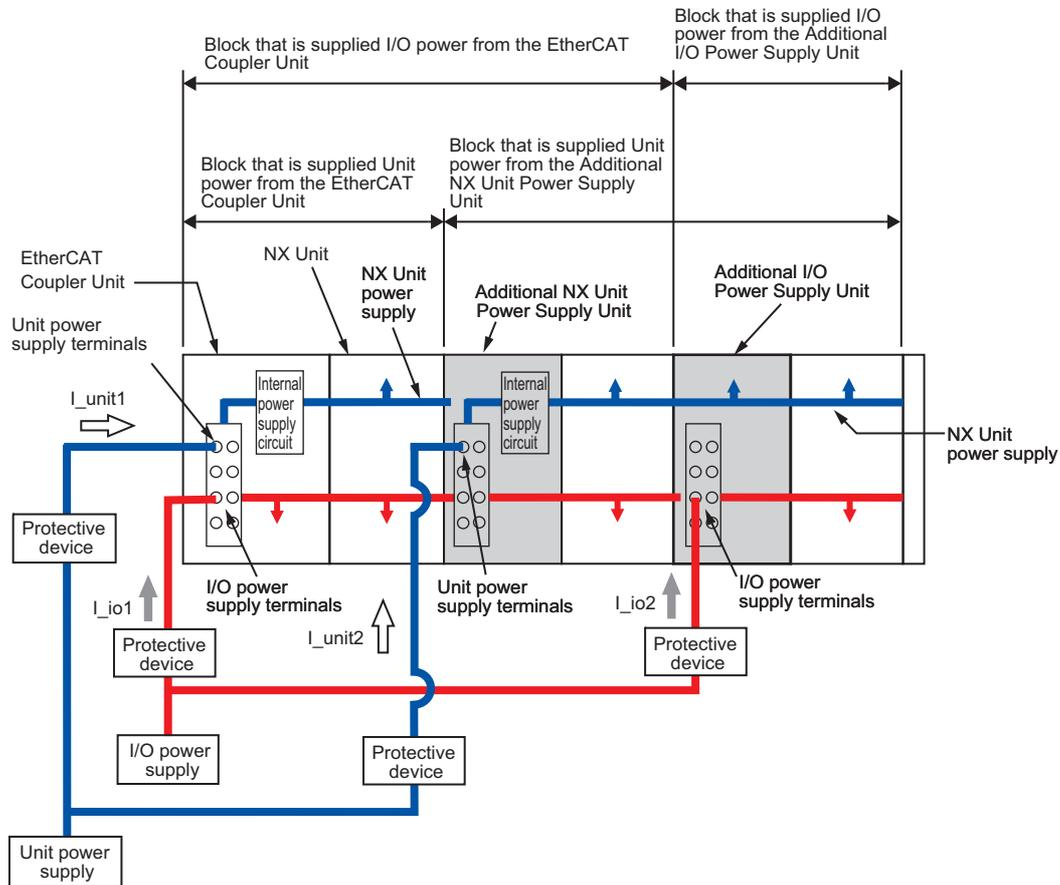
However, fewer protective devices may be required when the current consumption of each block does not exceed the rated current. An example of this is provided below.
