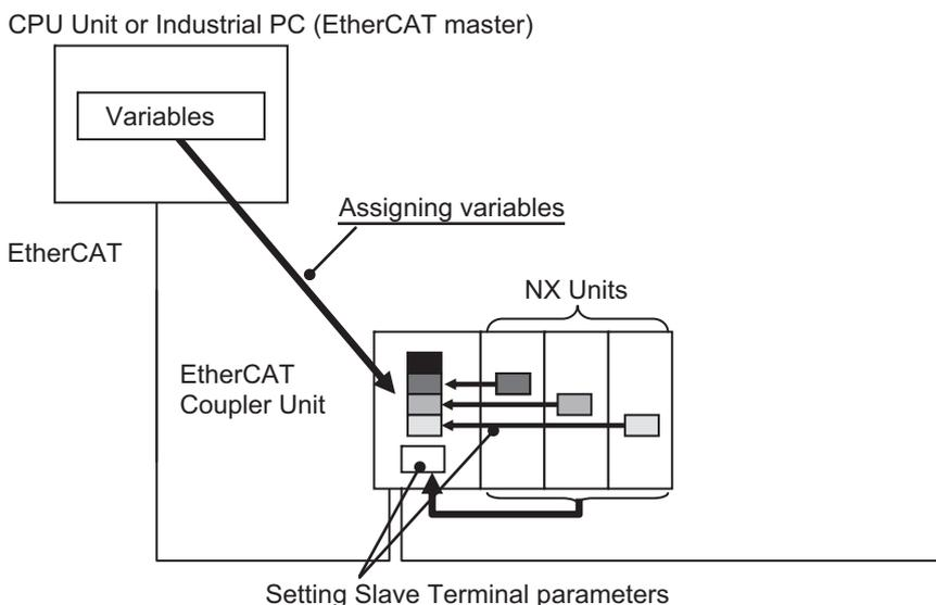
Make the above settings on the Sysmac Studio. Then connect the Sysmac Studio to the CPU Unit or Industrial PC and transfer the settings to the CPU Unit or Industrial PC and to the Slave Terminals.
