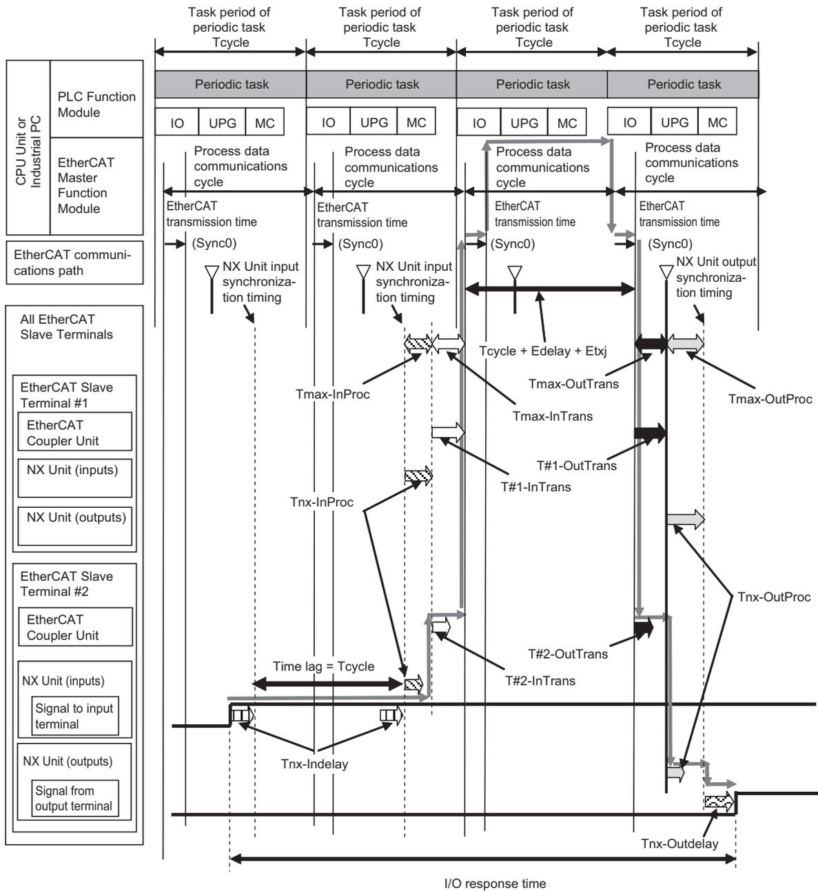
The maximum and minimum values of the I/O response time are calculated as shown below. The minimum value occurs when the time lag that is shown in the above figure does not occur.
