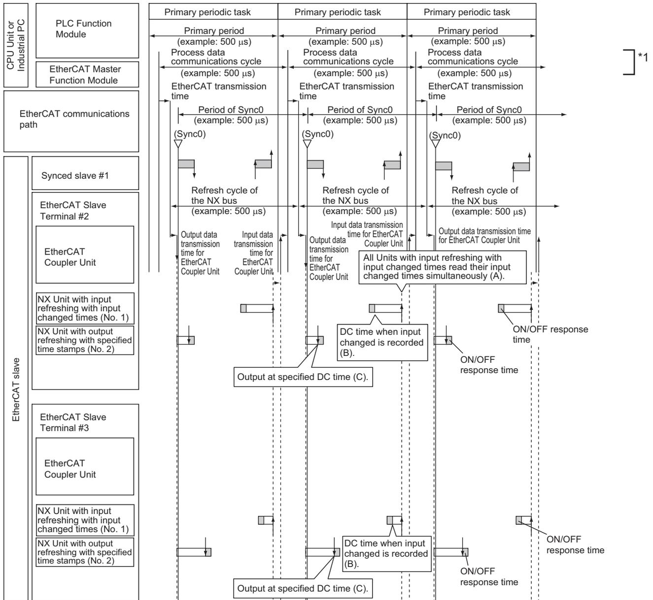
\*1. For a built-in EtherCAT port that can perform process data communications with a Slave Terminal in more than one periodic task, this is called process data communications cycle 1.
