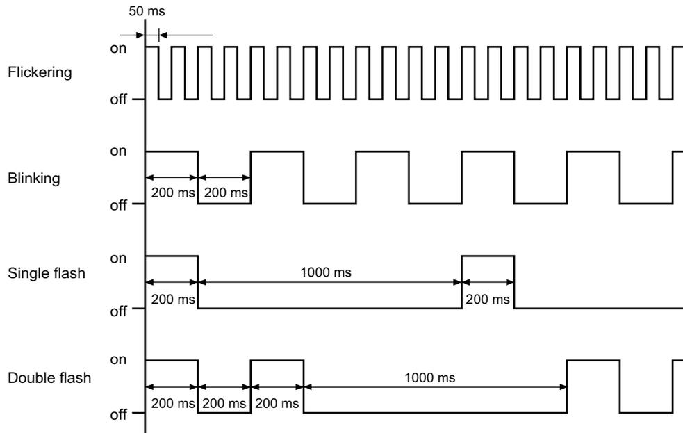
● **Troubleshooting the Primary Errors That Are Displayed with the UNIT PWR, L/A IN, L/A OUT, ERR, and TS Indicators**
