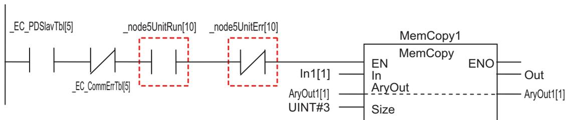
\* *\_node5UnitRun[10]*: This is a device variable for the EtherCAT Coupler Unit (with node address 5) to which the NX Unit I/O Data Active Status (NX Unit number 10) is assigned.
