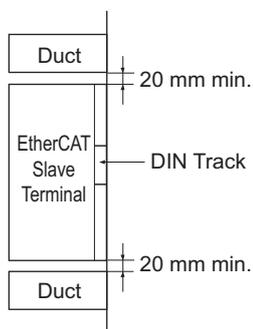
● **Wiring Duct Example**
