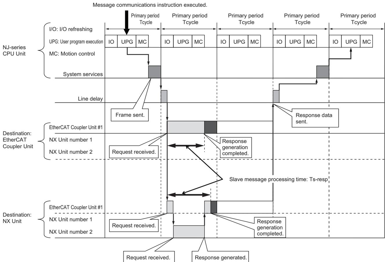
The definitions and values of  $T_{\text{s-resp}}$  are the same as the definitions and values for the calculation formula when connected to the built-in EtherCAT port on an NX-series CPU Unit.
