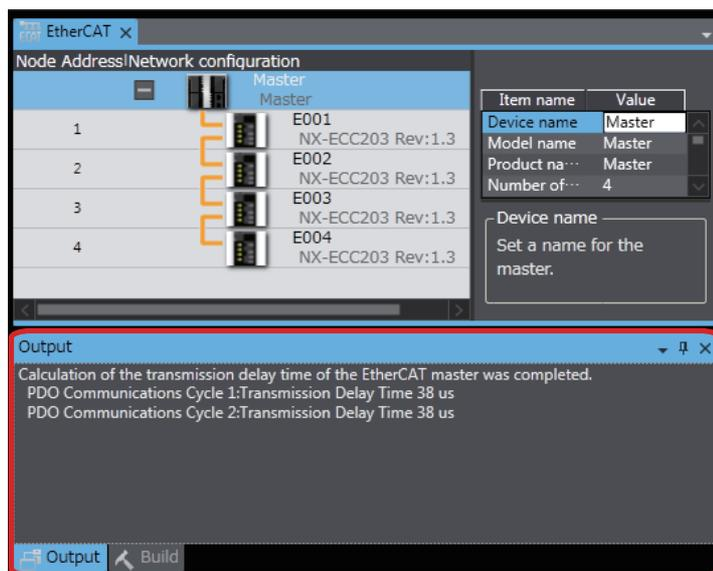
The transmission delay times of the EtherCAT master depend on the periodic tasks that are used in the CPU Unit or Industrial PC to refresh I/O for the EtherCAT Slave terminals, as shown below.
