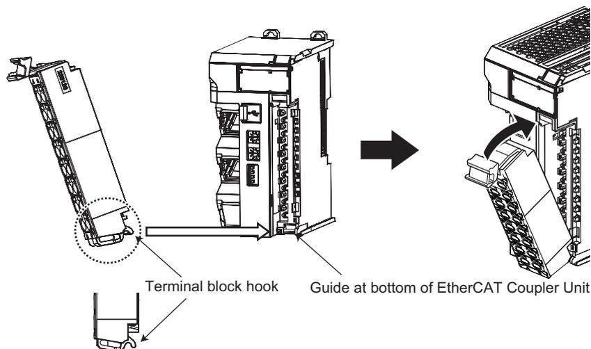
Mount a terminal block that is applicable to the model of the EtherCAT Coupler Unit.
