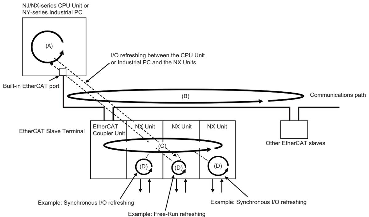
This section describes the operation of the NX Units on the EtherCAT Slave Terminals and the operation of I/O refreshing with the various series of CPU Units or Industrial PCs using the letters given in the above figure.
