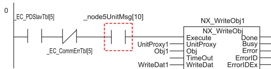
*\_node5UnitMsg[10]*: This is a device variable for the EtherCAT Coupler Unit (with node address 5) to which the NX Unit Message Enabled Status (NX Unit number 10) is assigned.
