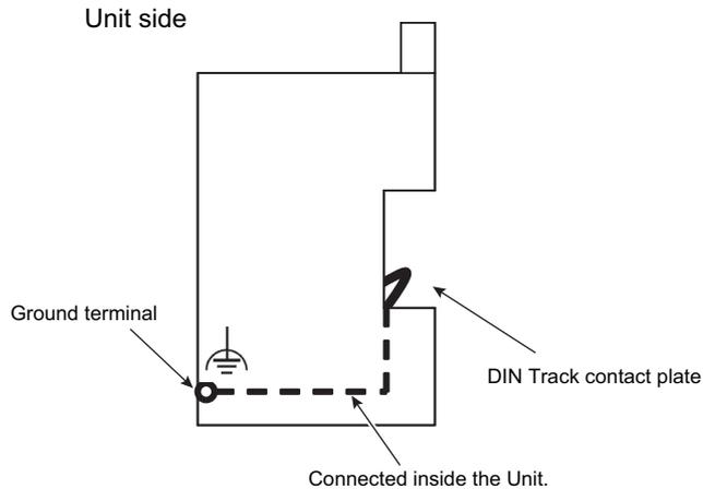
The DIN Track contact plate is connected internally to the ground terminal on the Unit.
