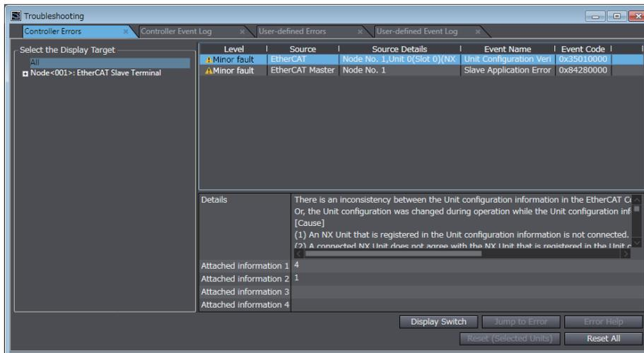
The current Controller errors are displayed on the Controller Errors Tab Page. (Observations and information are not displayed.)
