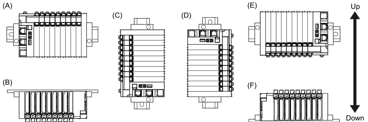
However, there are restrictions on the installation orientation of the EtherCAT Coupler Unit due to the ambient operating temperature and the NX Unit power supply capacity.
