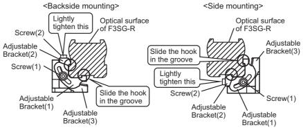
**4.** Adjust the Standard Adjustable Bracket to the mounting position of the wall surface. Securely tighten the Screw (2) to fix the Standard Adjustable Bracket to the housing of the F3SG-R. The recommended torque to tighten the Screw (2) is 2.0 N•m. (Fig. 3)
