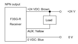
The load current of the auxiliary output is 100 mA max. (n)
