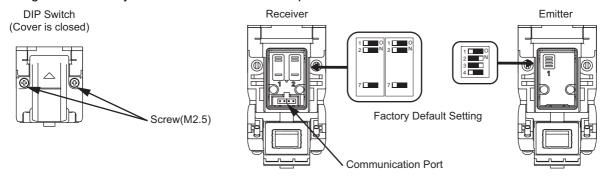
When attaching the cover, tightly fasten the screws (M2.5, recommended torque: 0.35N.m). Failure to do so may cause the cover to come loose, leading to deterioration of the protective functions. CHECK!
