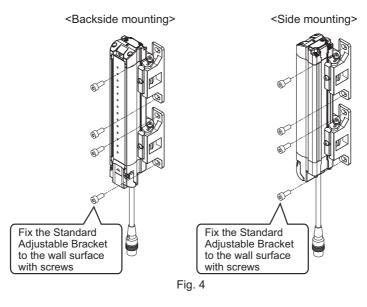
Screws to mount the brackets to the wall are not included.
