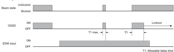
hapter2 External Device Monitoring (EDM)
