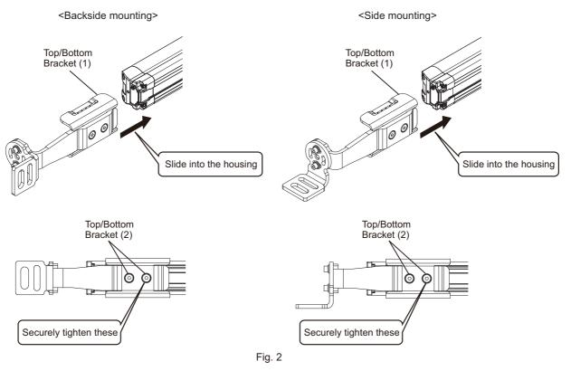
$\frac{1}{2}$  Tightening screws with a torque that considerably exceeds the recommended torque may cause failure.
