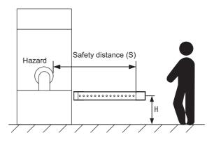
Also, you must include a hazardous condition under which a person may go through under a detection zone if H exceeds 300 mm (200 mm for other purpose than industrial use) into risk assessment.
