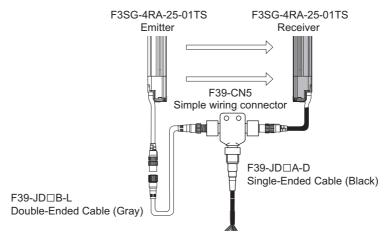
When using the Simple wiring connector (F39-CN5), the following functions are not available. • External Device Monitoring
