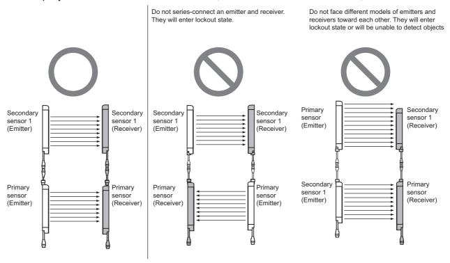
If caps and Cascading Cables are not connected properly, the F3SG-R enters lockout (when power is turned ON).
