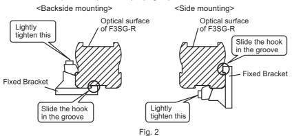
**3.** Adjust the Standard Fixed Bracket to the mounting position of the wall surface. Securely tighten the hexagon socket head cap screw (M3 x 15) to fix the Standard Fixed Bracket to the housing of the F3SG-R. The recommended torque to tighten the hexagon socket head cap screw (M3 x 15) is 2.0 N•m. (Fig. 3)
