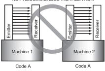
The scan code feature of the F3SG-R system allows for placement of systems in close proximity and in line with each other. The distinctive coding of the beams provide for unique operation of a system while in view of another system with a different scan code. Two unique codes are available on the F3SG-R.
