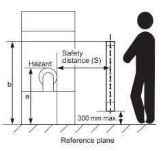
Note: Lower edge of the detection zone above 300 mm in relation to the reference plane does not offer sufficient protection against crawling below.
