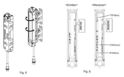
The angle adjustment range of the Standard Adjustable Brackets is ±15°.
