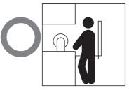
A person is between the sensor's detection zone and the hazardous zone of a machine.
