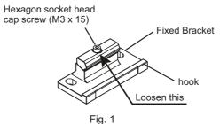
**2.** Slide the hook of the Fixed Bracket (1) in the groove of the F3SG-R housing. Lightly tighten the hexagon socket head cap screw (M3 x 15). (Fig. 2)
