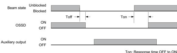
Ton: Response time OFF to ON Toff: Response time ON to OFF
