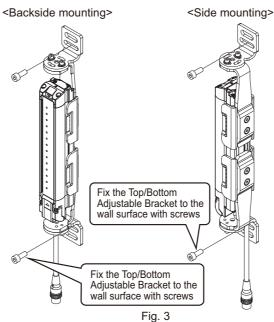
One screw at upper and lower positions, respectively, is sufficient to fix the F3SG-R to the wall surface. Screws to mount the brackets to the wall are not included.
