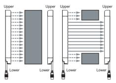
■ Response time of "OFF (Synchronized) → ON" and "OFF (Not synchronized) → ON" Response time of "OFF (Synchronized) → ON" is the response time from when the F3SG-R is in the OFF state and the emitter and receiver are synchronized to when the F3SG-R is turned to the ON state.
