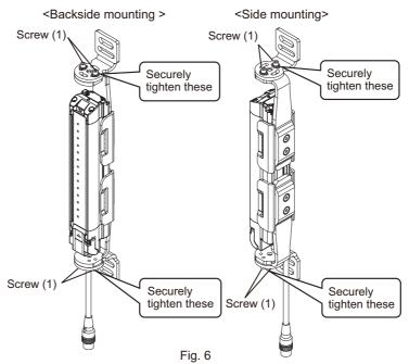
Tightening screws with a torque that considerably exceeds the recommended torque may cause failure.
