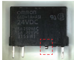
Deformation of the relay terminal
