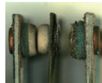
Corrosion due to nitric acid
