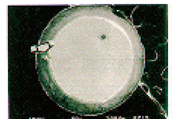
Magnified photograph of a diode short-circuit
