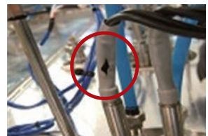
The area within the red circle is the location of the short-circuit.
