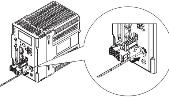
(3) Cleaning of the end face of the fiber connector of the sensor head side
