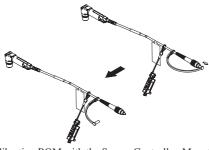
(2) Connect the fiber cable and calibration ROM with the Sensor Controller. Mount the fiber cable in the direction where the protruding portion of the fiber connector and the groove portion of the fiber adapter are aligned. Align the groove portion of the fiber adapter with the protruding portion of the fiber connector, and rotate the screw portion clockwise while pushing it.
