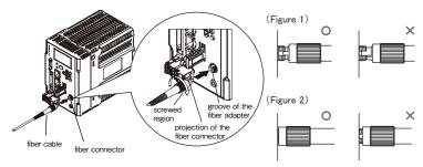
·If insertion of the fiber and tightening of the fixing screw shown as "x" on Fig. 1 and 2 are incomplete, the optical signal cannot be transmitted properly, resulting in incorrect measurement. Make sure that they are properly positioned as shown as "O" on Fig. 1 and 2.
