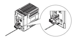
(3) Cleaning of the end face of the fiber connector of the sensor head side Remove the cap of the fiber connector, and wipe up and down the end face of the fiber around three times.
