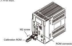
Before pushing in or pulling out the calibration ROM, be sure to turn off the power of the Sensor Controller. Otherwise, a failure might be caused
